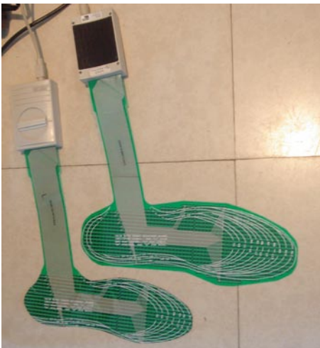
Fig. 18 Close-up of the pressure sensors of the Tekscan feeding signals to the computer
