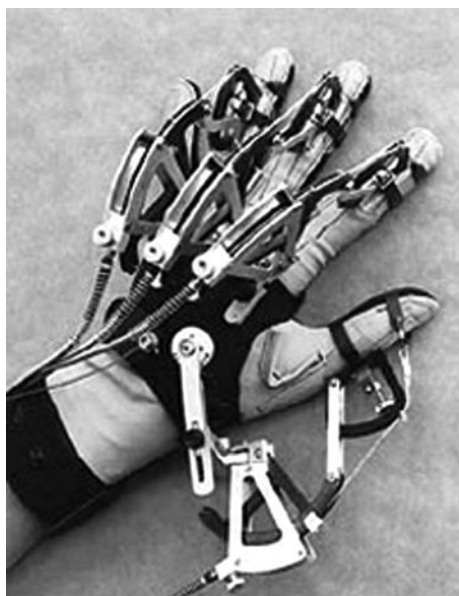
Fig. 51 The state-of-the-art CyberGrasp force feedback glove developed by the pioneering company immersion.com
