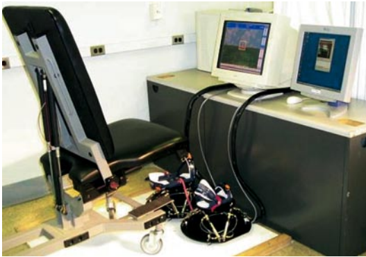
Fig. 65 Rehabilitation station including virtual reality simulation display and remote therapist communication console. © Rutgers University CAIP Center. Reprinted with permission
