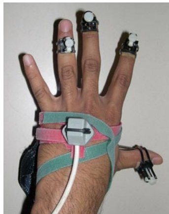
Fig. 62 The Rutgers Master II haptic glove used in hand rehabilitation, back view shows 3D tracker attachment. © Rutgers University CAIP Center. Reprinted with permission
