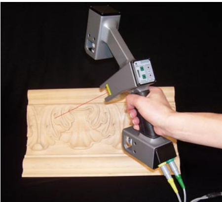
Fig. 48 An example of a 3D scanner marketed by Polhemus.com
