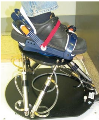
Fig. 64 The Rutgers ankle rehabilitation system: The pneumatic robot. © Rutgers University CAIP Center. Reprinted with permission
