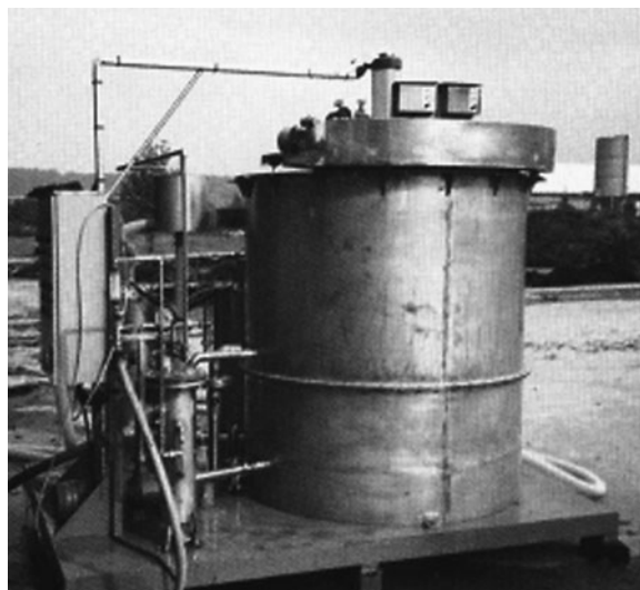
Fig. 9.5. The flotation/filtration cell (FF-cell) (35).
