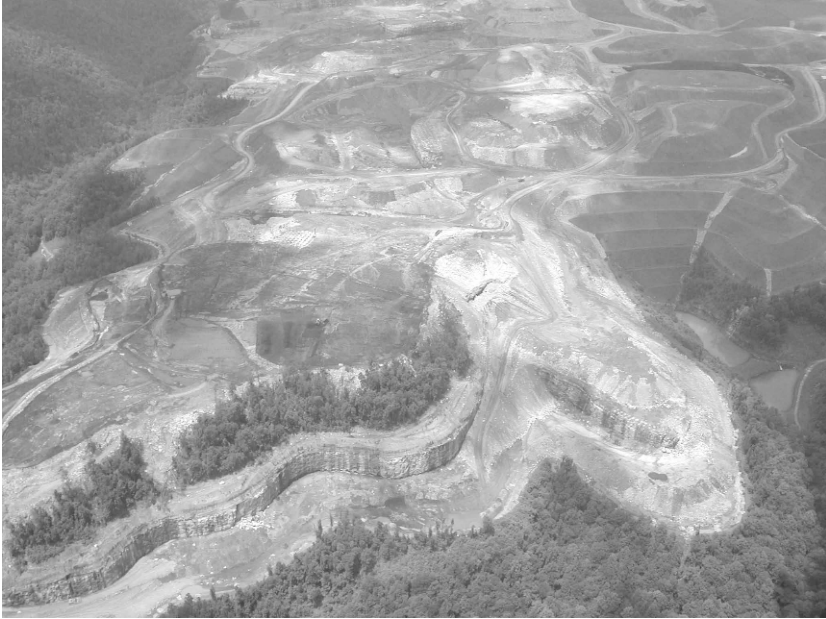
FIGURE 4-2. An example of mountaintop removal mining, southern West Virginia. (Source: Ohio Valley Environmental Coalition. Photo credit: Vivian Stockman. Flyover courtesy: SouthWings.org.)
