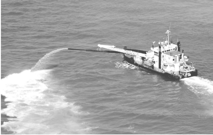
FIGURE 4-1. The Merritt , a sidecaster in the Corps' Wilmington District. (Source: U.S. Army Corps of Engineers.)
