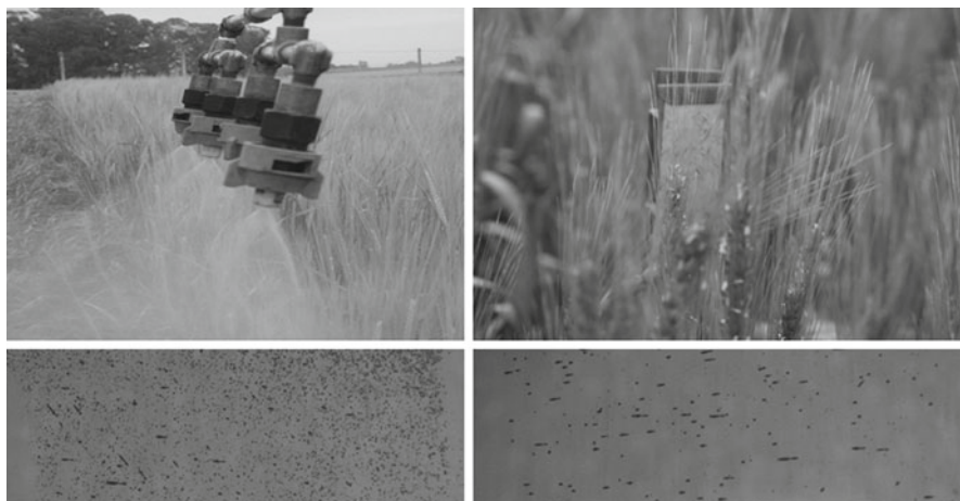
Fig. 11.3 ConeJet 03 nozzles, water sensitive cards located in the middle of the plot, forward support ( left ), back support ( right )
