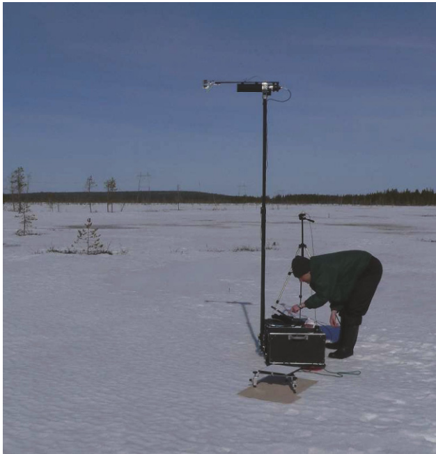
Fig. 9.3. The FIGIFIGO measuring BRF and polarization in Sodankylä in 2009. Optics is located horizontally in the upper end of the arm, and is looking down to the target through a mirror. The mirror has two small actuators to fine tune the spot location or scan over a small range. In front is the Spectralon white reference target, and behind the researcher’s head is the sun and sky light monitoring pyranometer.
