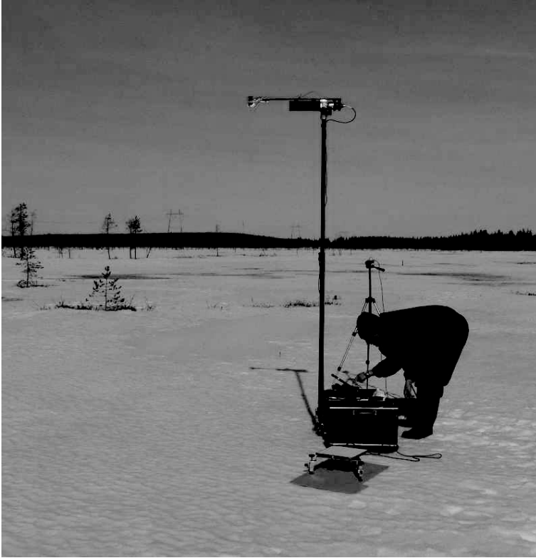
Fig. 9.3. The FIGIFIGO measuring BRF and polarization in Sodankylä in 2009. Optics is located horizontally in the upper end of the arm, and is looking down to the target through a mirror. The mirror has two small actuators to fine tune the spot location or scan over a small range. In front is the Spectralon white reference target, and behind the researcher's head is the sun and sky light monitoring pyranometer. [For a color version of this figure, see the color section.]
