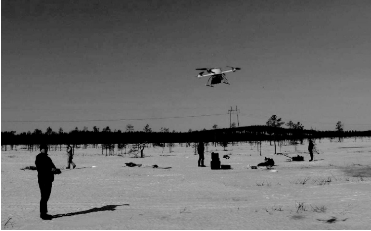
Fig. 9.29. Experimenting with BRF measurements simultaneously using FIGIFIGO (on the right of the background) and Microdrone md4-200 UAV with Ricoh GR II digital camera. The pilot stands on the left of the foreground, and in the middle of the background is another spectral measurement going on. [For a color version of this figure, see the color section.]
