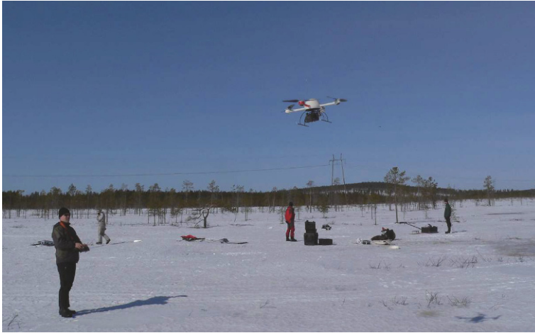
Fig. 9.29. Experimenting with BRF measurements simultaneously using FIGIFIGO (on the right of the background) and Microdrone md4-200 UAV with Ricoh GR II digital camera. The pilot stands on the left of the foreground, and in the middle of the background is another spectral measurement going on.
