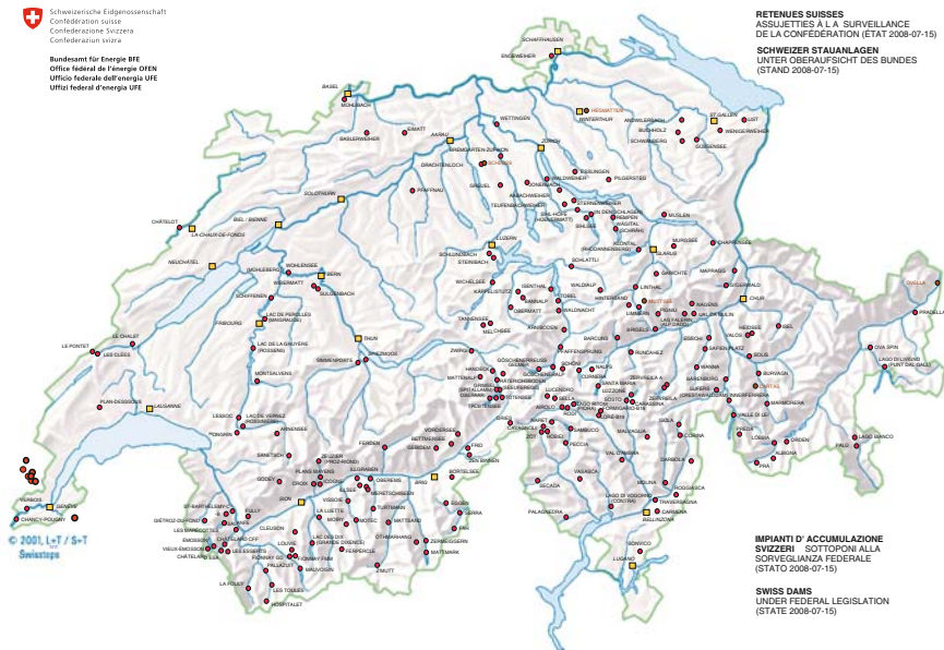
Fig. 3 Map showing the location of the 220 largest dams in Switzerland. The reservoirs have an integrated storage of more than 4 \text{ km}^3 and provide a typical annual power production of 38 TWh. As the map indicates, basically all major alpine rivers are affected by abstraction or hydro-peaking
