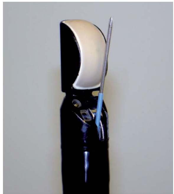
Fig. 12.1 Linear-array echoendoscope with 19-gauge needle.
