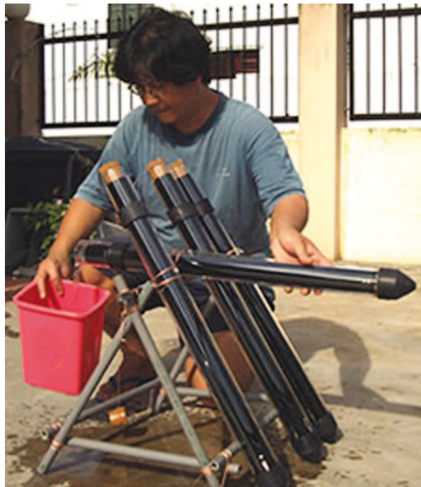
Fig. 3.6 An array of Solar Kettles articulated to pour out the pasteurized water. (Photo credit: Alex Kee)
