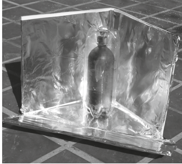
Fig. 3.7 A black 1 l PET bottle inside a cover made from two 2 l PET bottles (Bottle 2, Cover 2); the reflector in front is tilted up. (Photo credit: Ed Pejack)
