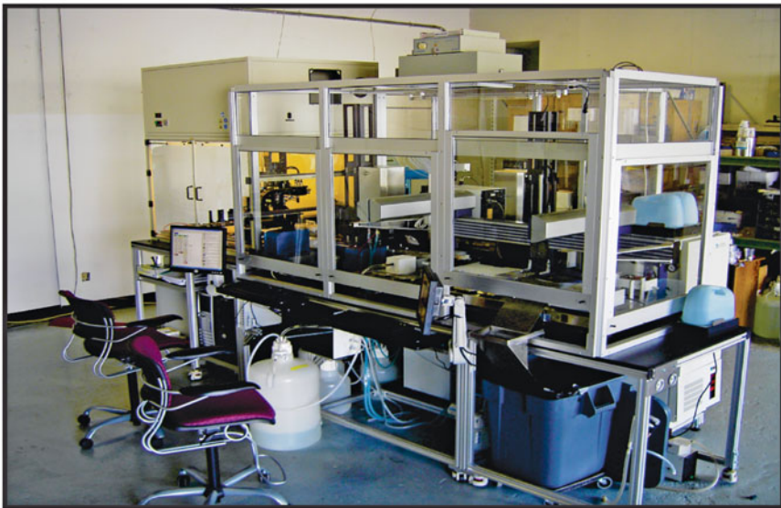
Fig. 1 Schematic and picture of integrated robotic workcell. SoftLink-scheduled, advanced integrated workcell to fully automate high-throughput molecular biology routines and perform high-content screening. 1A Track 1, 1B Track 2, 2A StackLink (Track 1), 2B StackLink (Track 2), 3 4-Axis PlateCrane EX, 4 Colony Picker/Arrayer, 5 PCR Thermal Cycler with Autolid, 6 UV/VIS Plate Reader, 7 ABgenePlate Sealer (foil), 8 Plate Sealer (porous tape), 9 Liquid Handler with Centrifuge, 10 Hudson Micro10 Filler, 11 Hudson Plate Aspirator, 12 Automated Incubator, 13 Passive Stackers, 14 Computer and Monitor, 15 Barcode Reader, S1–S6 StopLink Plate Positions, StopLink Plate
