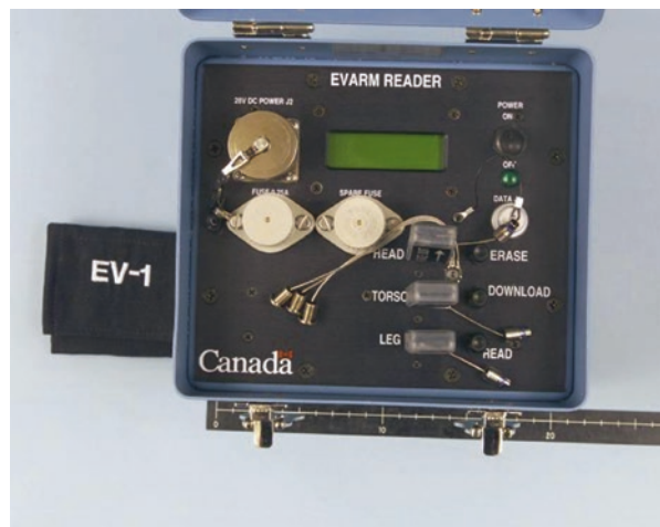
Fig. 5.1 A Canadian Space Agency radiation dosimeter used during spacewalks. (Image courtesy of CSA)
