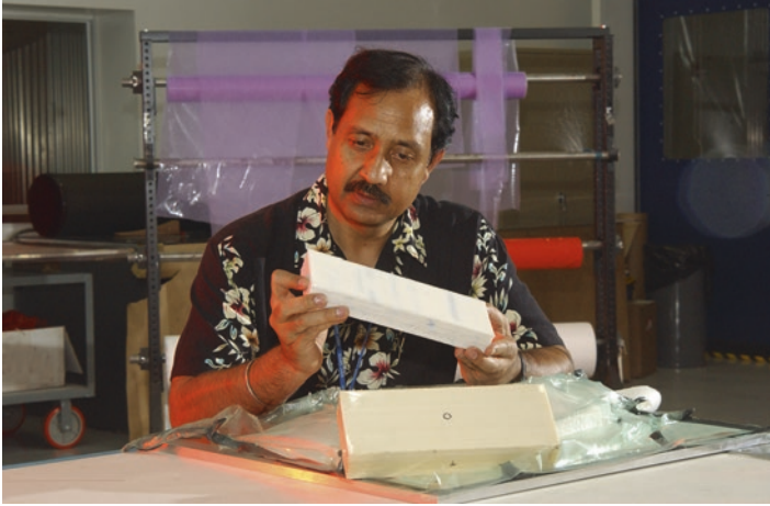
Fig. 6.8 Dr. Raj Kaul examines “bricks” of radiation shielding material made in his composites laboratory at NASA’s Marshall Space Flight Center in Huntsville, AL. Kaul has investigated the effectiveness of material used to shield spacecraft from radiation. (Image courtesy of NASA/MSFC/Doug Stoffer)
