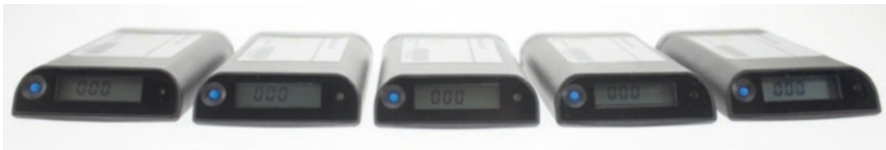
Fig. 5.5 Wearable units of the new European crew personal active dosimeter—EuCPAD—system for active radiation monitoring of astronauts in orbit. (Image courtesy of NASA)
