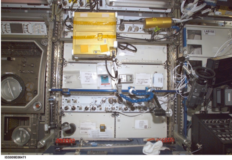
Fig. 5.3 EXPRESS Rack 5 with the intravehicular charged particle directional spectrometer (IV-CPDS) (gold box in left field of view), Tissue equivalent proportional counter (TEPC) radiation detector (gold cylinder) and upper storage compartments visible. EXPRESS Rack 5 is in the Destiny/U.S. laboratory. Image taken during Expedition 9. (Image courtesy of NASA)
