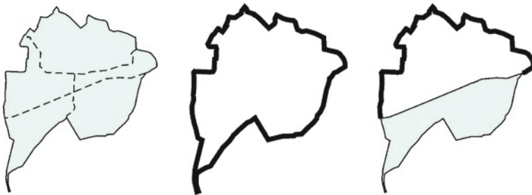
Fig. 28.2 Illustration of alternatives 0 (left), 1 (middle) and 2 (right). The bold lines indicate the location of overtoppable dikes
