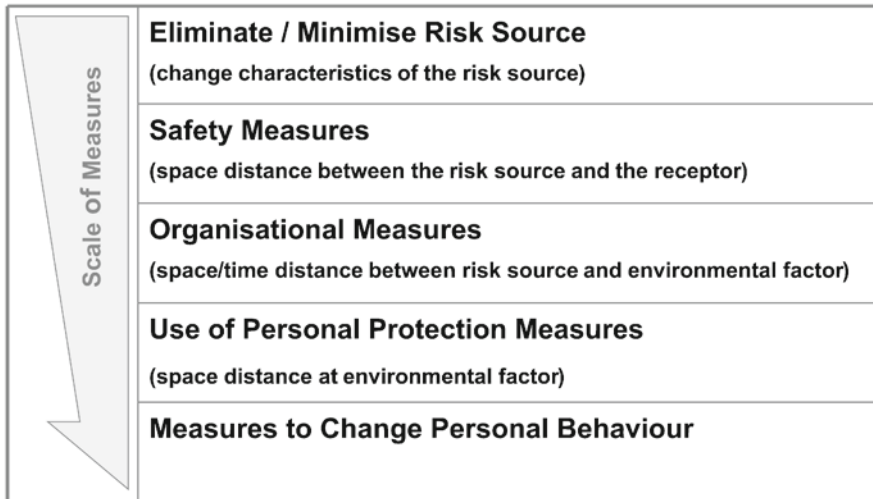
Fig. 31.4 Type and hierarchy of basic types of measures, evaluated for climate change adaptation measures
