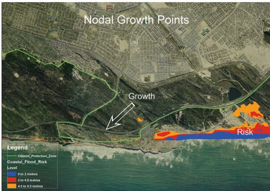
Fig. 32.3 The CPZ overlaid with the coastal inundation risk model. Appropriate areas have been identified for future nodal development
