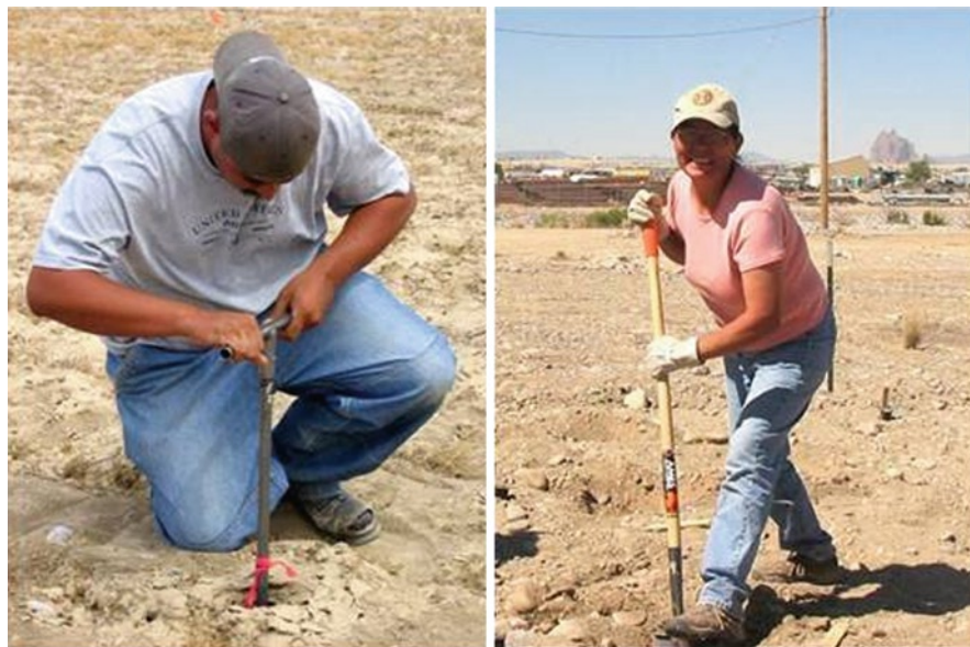
Fig. 6.6 Diné College students Thoe Peterman and Beverly Maxwell sampling soils for physical and chemical properties, and transplanting native phreatophytes to establish phytoremediation test plots at Shiprock, New Mexico
