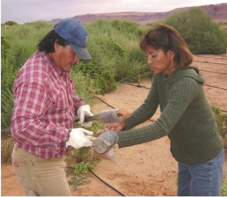
Fig. 6.4 Diné College students Garry Jay and Rita White sampling soil for nitrogen content as part of soil and groundwater phytoremediation pilot studies at Monument Valley, Arizona
