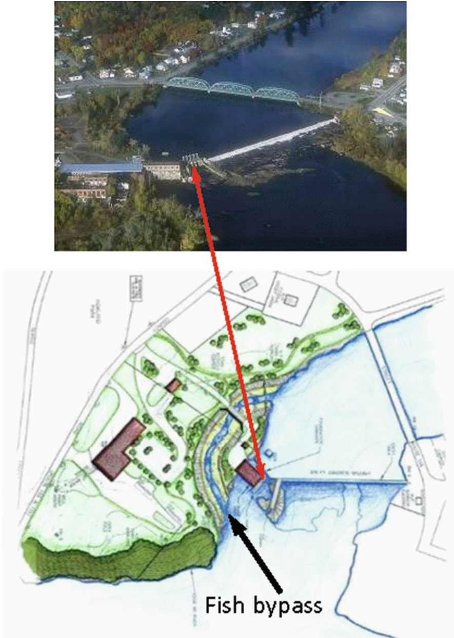
Fig. 13.4 The design for the fish bypass at Howland Dam, seen in photo. The red arrows point to the same structure in each image. The black arrow points to the downstream entrance to the fish bypass (images courtesy of MMI engineering)
