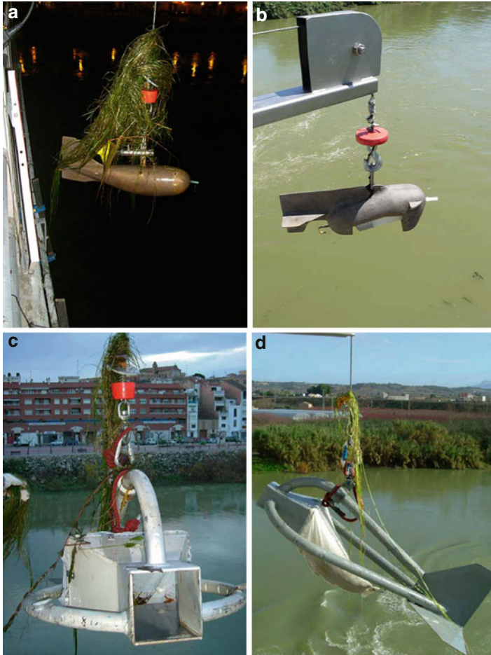
Fig. 2 Cable suspended sediment samplers in operation at MEMS (Fig. 1), lower Ebro, during floods: (a) US DH-74 depth-integrating suspended sediment sampler; (b) US DH-59 depth-integrating suspended sediment sampler; (c) 152 mm intake Helley–Smith sampler; (d) 76 mm intake Helley–Smith sampler. See text and [25] and [31] for operational details
