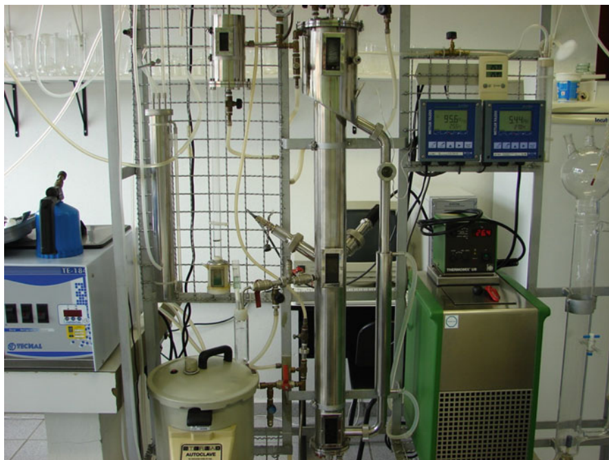
Fig. 1 Pneumatic (5 L) airlift bioreactor (Rossi et al. submitted )
