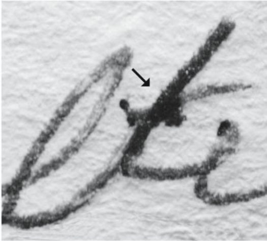
Fig. 13.3. Patched writing showing that a writer wrote over an existing line to improve its appearance. Forgers patch their work to improve its appearance.
