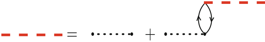
Fig. 12.7 Diagrammatic expression of Dyson equation for the effective Coulomb propagator W = V + V\Pi_0 W with \Pi_0 = -\chi_0
