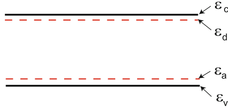
Fig. 7.3 Impurity levels in semiconductors doped with N_d donors and N_a acceptors per unit volume
