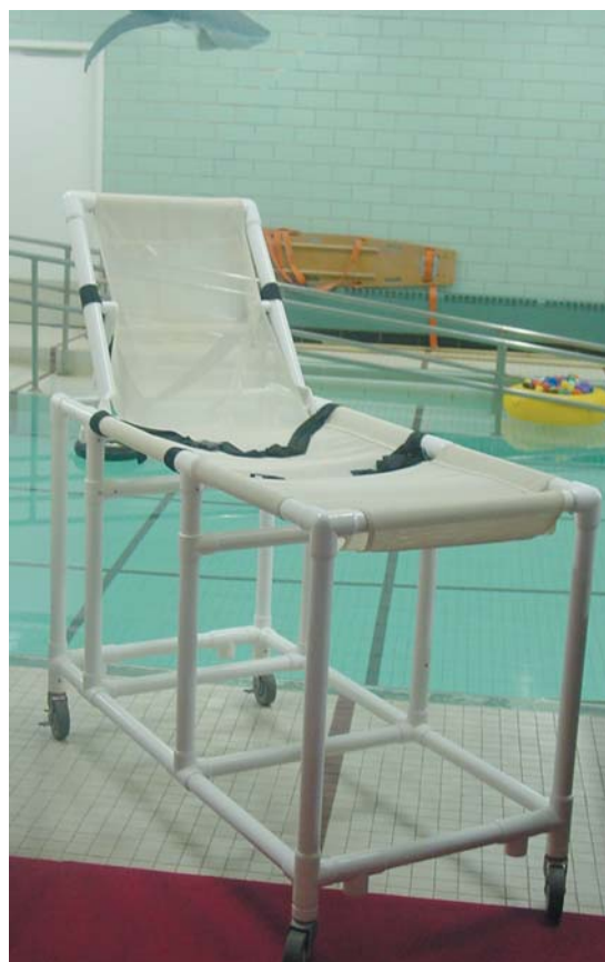
Figure R4. One problem in doing hydrotherapy for large individuals who are totally dependent for dressing and movement is finding changing rooms or tables. Low-cost solutions can easily be developed using construction and plumbing supplies. A volunteer for the school constructed this changing table.
