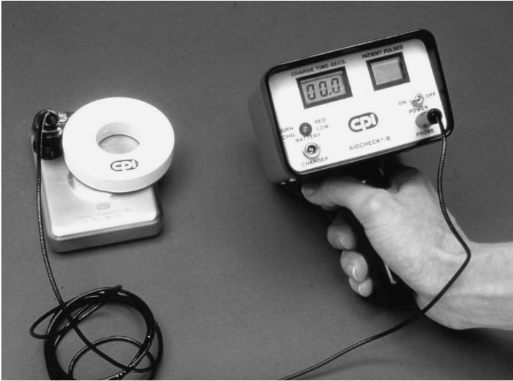
FIGURE 1.1. Read-out of the device, using a doughnut-magnet, which allowed capacitor reformation. Via audible tones synchronicity with the R-wave was assessed (AID and AICD, Intec; later Ventak 1500 series, CPI).
