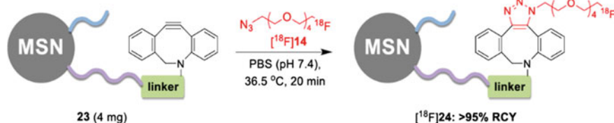
Fig. 14.2 Formation of ^{18}\text{F} -labeled ADIBOT-PEG-MSNs under physiologically similar conditions (pH 7.4, 36.5 °C) in PBS by SPAAC reaction of ADIBO-PEG-MSNs with ^{18}\text{F} -labeled azide. Adapted from [39] with permission
