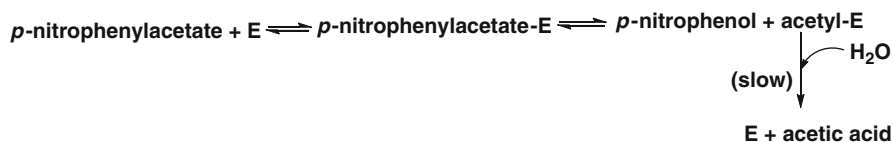
Fig. 4.26 All steps in the conversion of p -nitrophenylacetate to p -nitrophenol and acetate-E are rapid. The rate-limiting step in the chymotrypsin reaction is the dissociation of acetic acid from the enzyme
