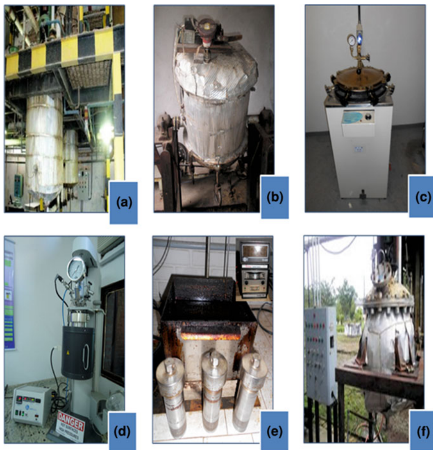
Fig. 2.3 Systems explored for dilute acid hydrolysis of various agro-residues at Engineering School of Lorena (EEL), University of Sao Paulo, Lorena. a Large reactor of capacity 1,000 L. b Medium size rotator reactor. c Autoclave equipped for acid hydrolysis of biomass. d Parr reactor. e Oil bath reactor with stainless steel made hydrolytic vessels. f Medium size static reactor
