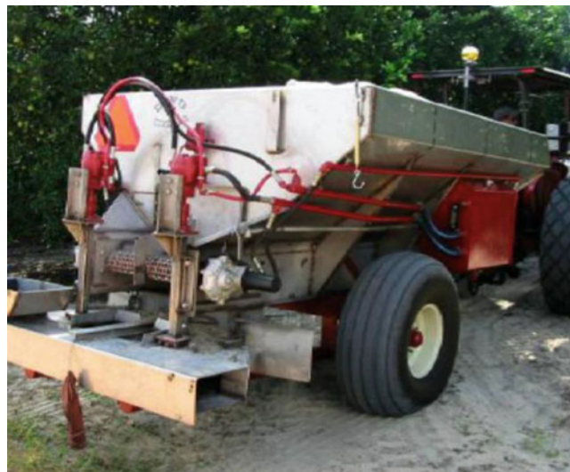
Fig. 26.2 Smart spreader uses infrared or ultrasonic sensors to sense tree and adjust the speed of the application chains that deliver the fertilizer to the fans. In areas where trees are small or weaker, less fertilizer is used, saving money and wasted fertilizers
