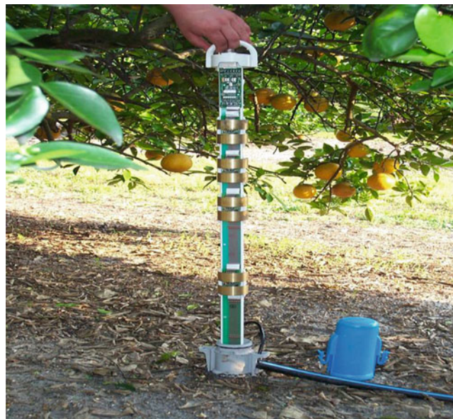
Fig. 26.3 Multisensor capacitance probe installed in access tube in citrus orchard
