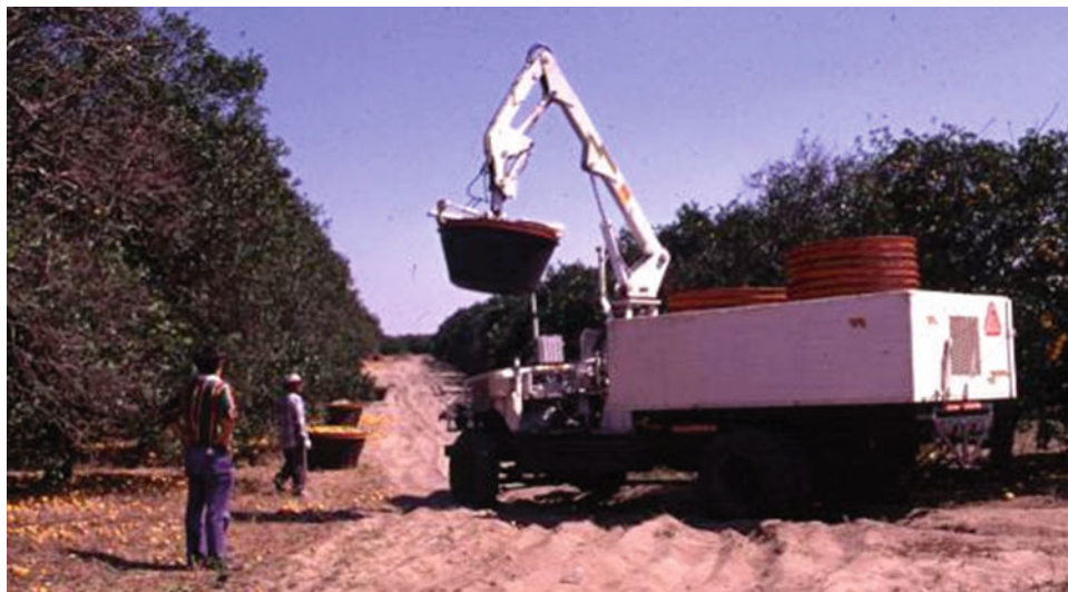
Fig. 18.3 An instrumented truck equipped with a GeoFocus Goat GPS (yield monitor) used in collecting manually harvested citrus field tubs
