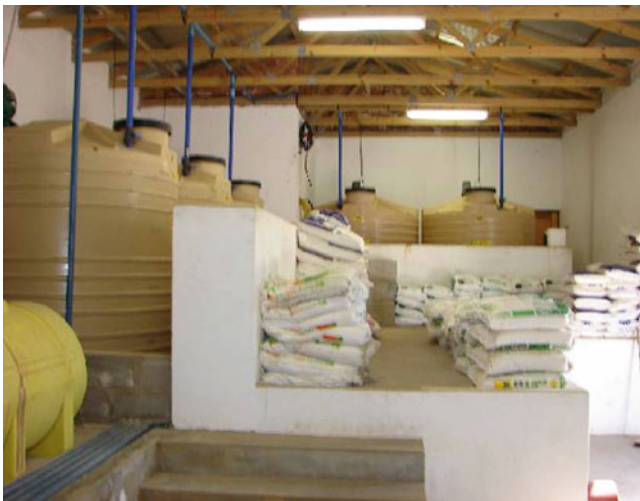
Fig. 19.6 Fertilizers can be custom blended using dry materials and multiple storage tanks connected to the fertigation system (Photo by K. T. Morgan)
