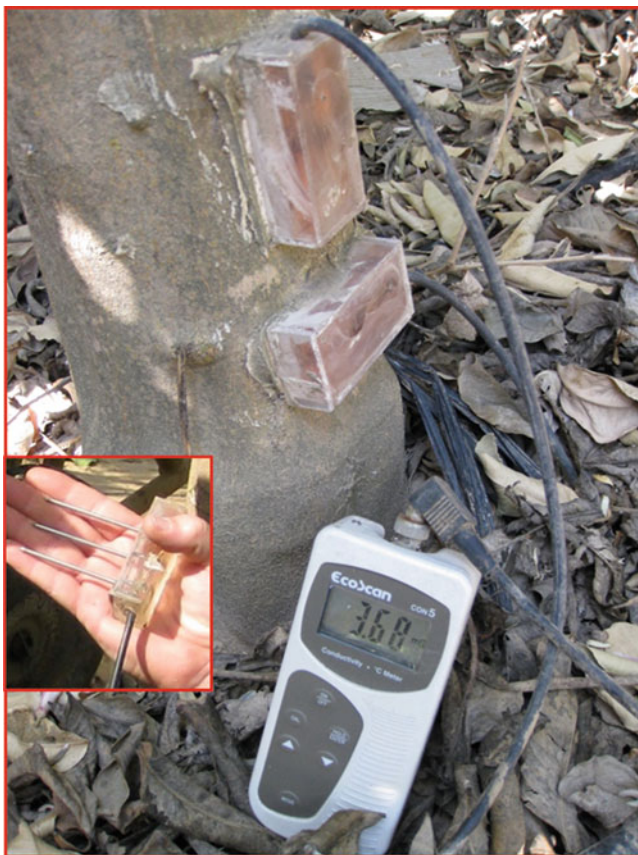
Fig. 28.6 The probes used for stem water content measurement in a pomelo trees ( Citrus maxima × Citrus grandis ). The probe can be connected to a TDR or to an EC meter (as seen in the picture). At the bottom, we can see the probe with the rods before it was installed to the main stem of the tree. The steel rods are 7 cm in length and can cross the stem from side to side (Picture by E. Raveh and A. Nadler)
