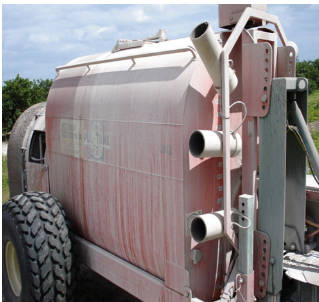
Fig. 26.1 Airblast sprayer equipment with sensors for turning nozzles on when a tree is detected
