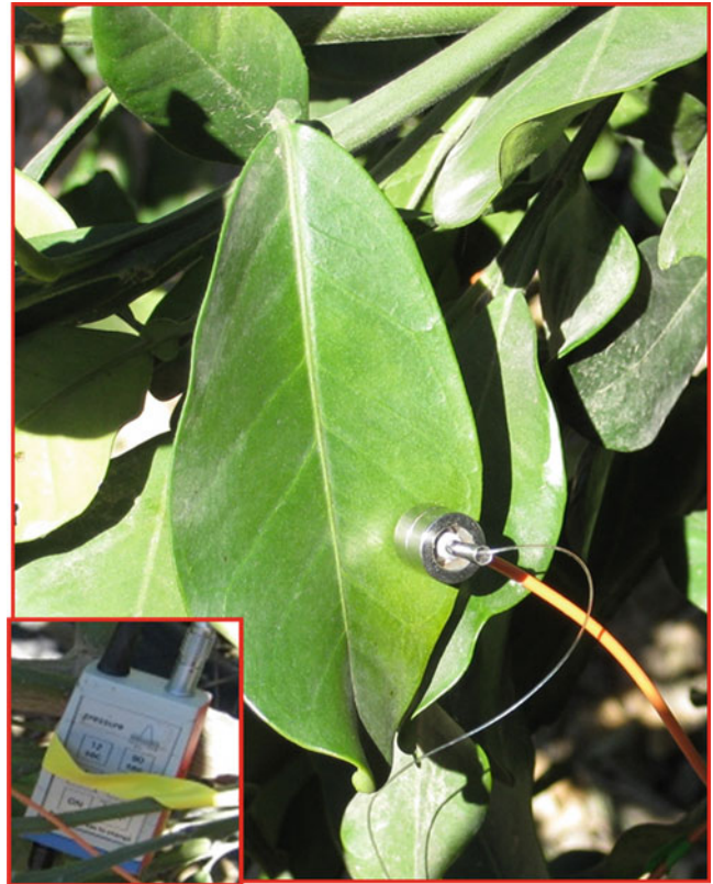
Fig. 28.7 The leaf patch clamp pressure (LPCP) probe used by Rüger et al. (2010) for measurement changes in tree water status in pomelo trees ( Citrus maxima × Citrus grandis ). At the bottom, we can see the transmission unit that connected directly (by the orange cable) to the probe and used for sending data to the main system (Picture by E. Raveh and Z. Hillman-Bronshtain)
