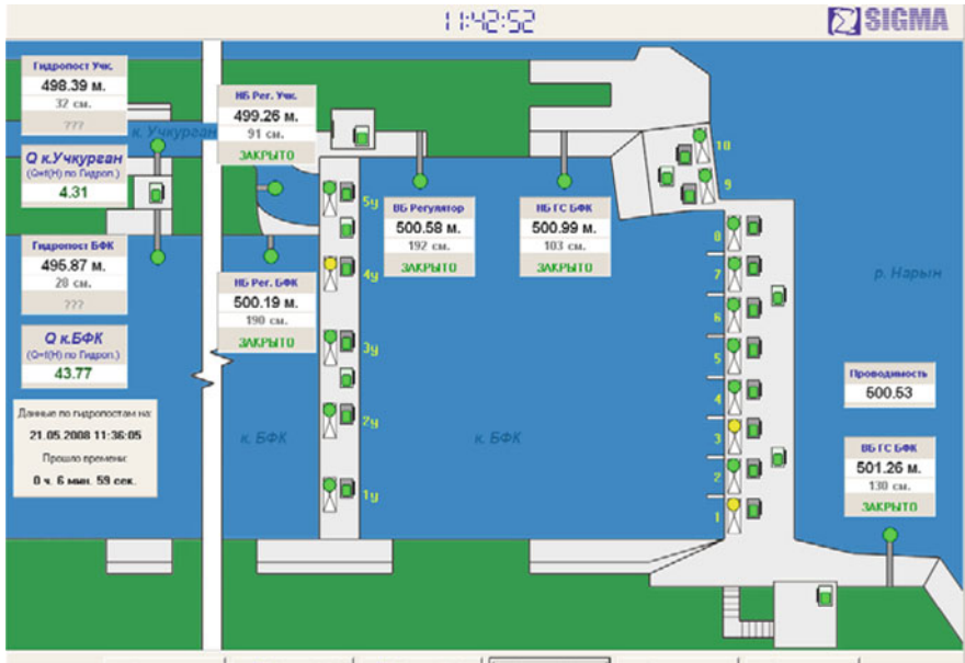
Fig. 4 Main symbolic circuit of the system of automation and controlling of the BFC headworks
