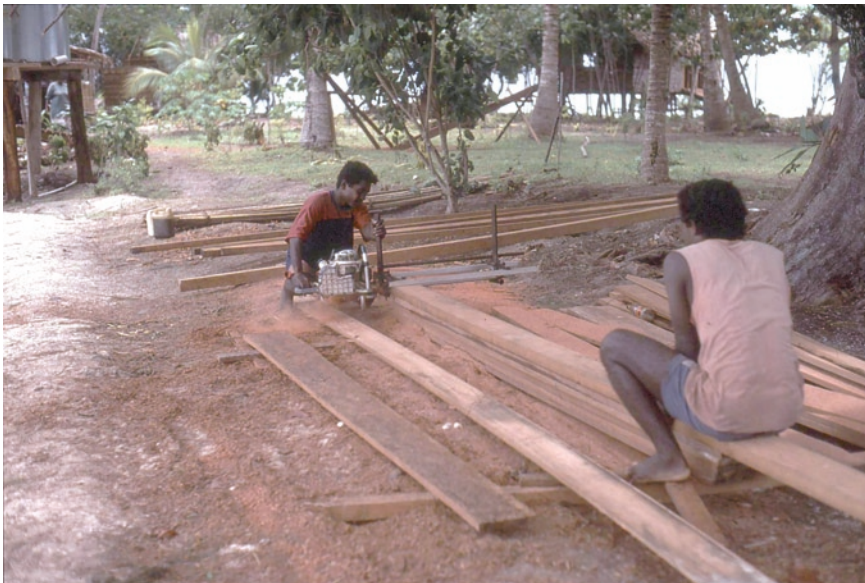
Fig. 3.2 Sawn timber being produced using a chain saw and a portable frame in Solomon Islands. This allows traditional forest owners to produce boards and fitches from their own logs and so increase their income
