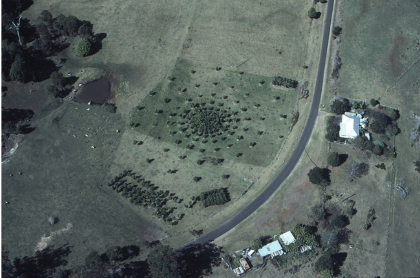
Fig. 6.9 A Nelder wheel layout for examining the effect of tree spacing on tree growth and morphology. The average area per tree is smaller (and hence the tree density is higher) in the inner rings of the trial than in the outer rings
