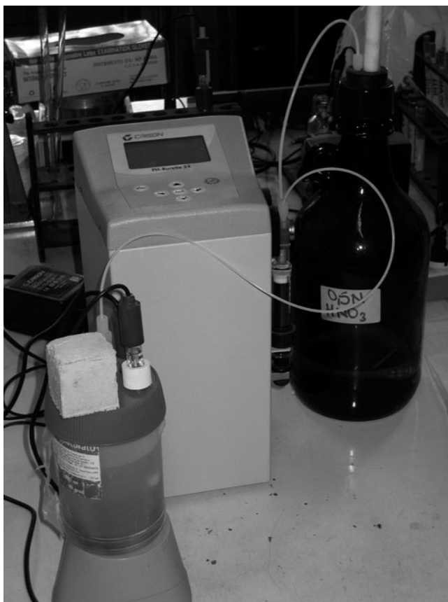
Fig. 10.1 Apparatus used for the monolith leaching test
