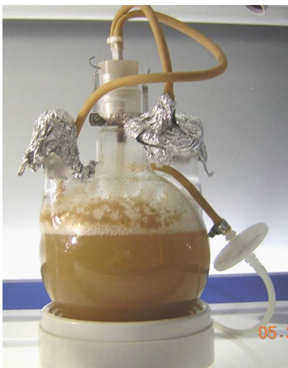
Fig. 24 A 3 L aerated bioreactor containing cell suspension culture
