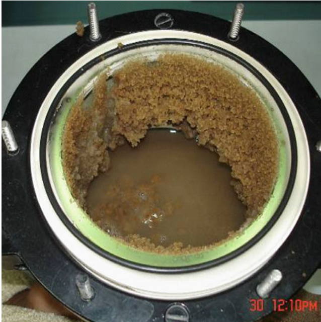
Fig. 26 Stirred tank bioreactor showing growth of cells for harvest
