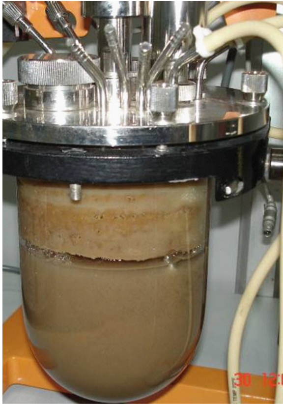
Fig. 25 A 2L stirred tank bioreactor with cells
