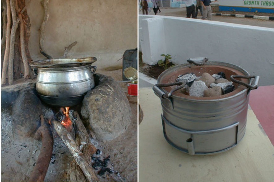
Fig. 1.1 A traditional three stone stove ( left ) and a charcoal stove ( right ) (Source: Ballard-Tremer)
