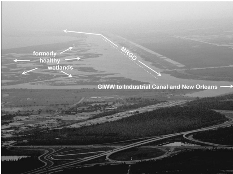
Aerial view of GIWW (narrower channel, running left-right) and MRGO “funnel,” looking toward the south, as taken in the fall of 2007. The dotted line indicates the approximate initial width of MRGO channel, which along this stretch had eroded to become more than half a mile wide by the time of Hurricane Katrina. Photograph by Robert Gramling.
