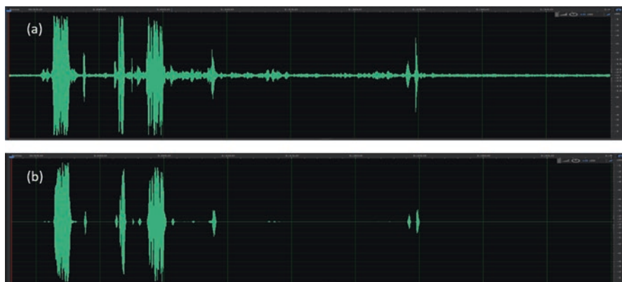
Fig. 6.12 (a) Original signal and (b) signal with automatic gain control (AGC) set for gain expansion (overall duration 55 s)
