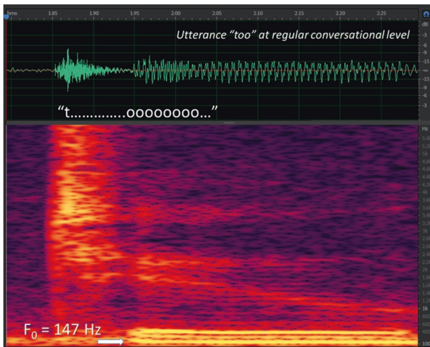
Fig. 9.25 A recording of a male talker uttering the word “too” at a normal conversational level of vocal effort (overall duration 0.5 s, frequency range 100 Hz–5.6 kHz, linear scale)
