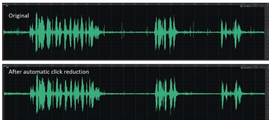
Fig. 6.16 Software detection and reduction of clicks in an audio recording (overall duration 11 s)
