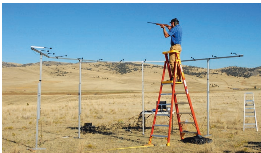
Fig. 9.11 Research recording setup used to obtain quasi-anechoic gunshot data for 12 azimuths from 0 to 180°. The marksman's head, arms, and torso cause natural reflections and diffraction, especially for the microphones located at the azimuths 90–180°. The firearm and the microphones are elevated so that the full duration of the muzzle blast can be recorded prior to the arrival of the first major reflection from the ground (Routh and Maher 2016)
