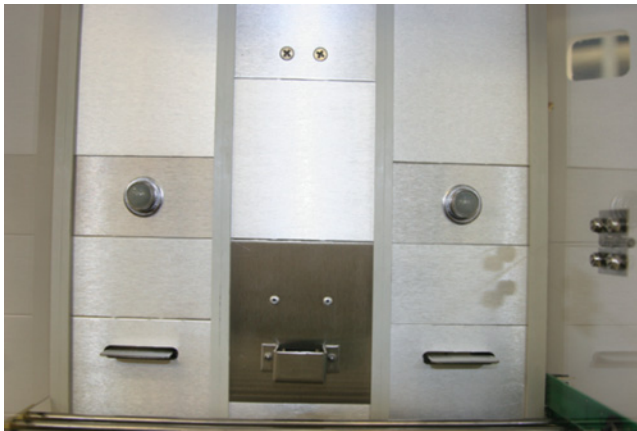
Figure 2-2. An inside view of a typical (and basic) operant chamber, used for drug discrimination studies, that consists of two levers and a device centered between the levers for the presentation of reinforcement (inside lights may or may not be present). Pressing of a bar produces the presentation of reinforcement. Photo courtesy of Coulbourn Instruments.
