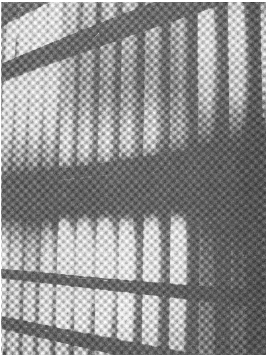
Figure 6. Color variation along the length of single halophosphor “cool white” fluorescent lamps (personal communication).
