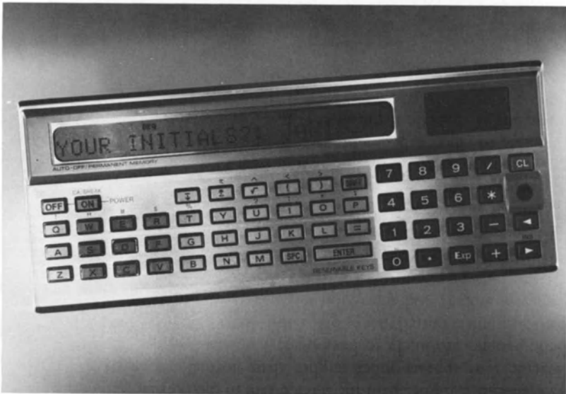
Figure 3-3. The hand-held computer for suggesting insulin adjustments.
