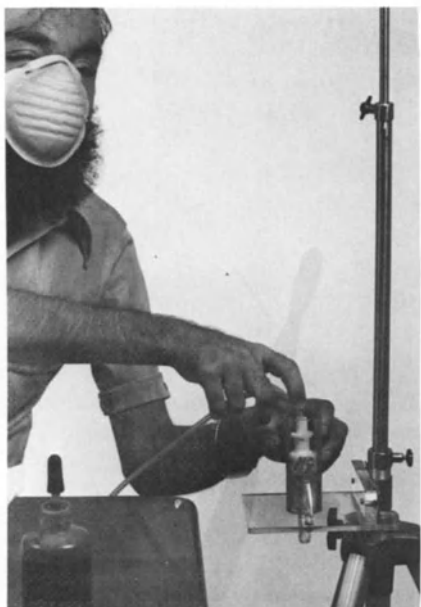
a) Insert spike coupler in the hole of the special tray with guide.
