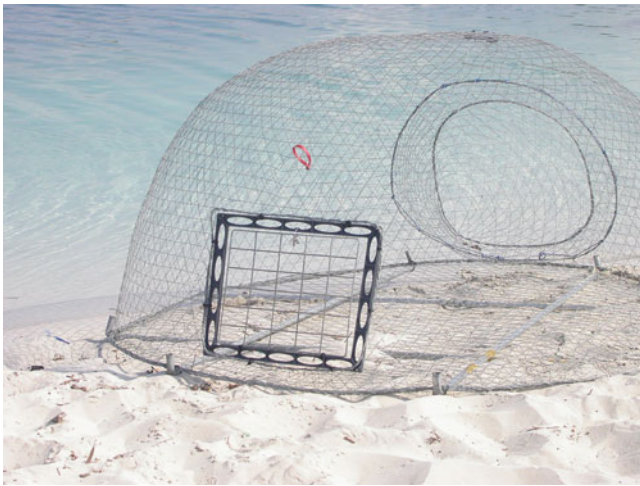
Fig. 8.33 A typical wire trap used to exploit reef fish in the Gulf. The escape panel is held shut with a magnesium zinc alloy pin which corrodes after 2 weeks, opening the panel so trapped fish can escape. In addition to the prevention of ‘ghost fishing’ the larger mesh on the escape panel was intended to mitigate the retention of juvenile fish (Photo: S. Hartmann)
