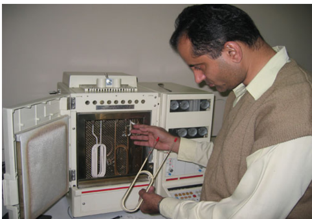
Fig. 3 Columns containing stationary phases are installed in GC
