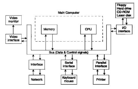
Fig. 11.1. Basic components of a computer.
