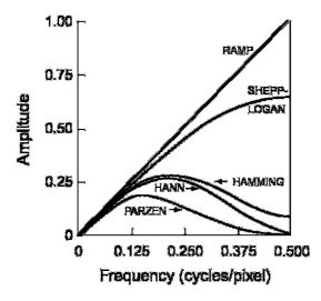
Fig. 12.10. Different filters for SPECT that are obtained by multiplying the respective windows by the ramp filter with cutoff at Nyquist frequency of 0.5 cycle/pixel.
