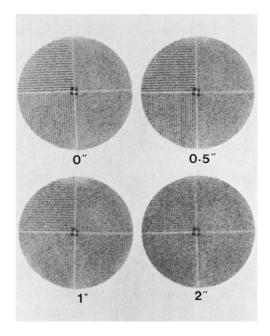
Fig. 10.4. Bar phantom images at different distances from a parallel-hole collimator.
