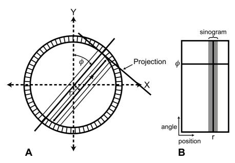
Fig. 13.6. PET data acquisition in the form of a sinogram. (A) Each LOR datum is plotted in  $(r, \phi)$  coordinates. (B) Data for all r and  $\phi$  values are plotted to yield the sinogram indicated by the shaded area (only a part is shown). (Reprinted with the permission of the Cleveland Clinic Foundation.)
