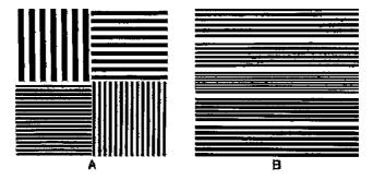
Fig. 10.3. (A) Bar phantom. (B) Hine–Duley phantom. (Courtesy of Nuclear Associates, Carle Place, NY.)
