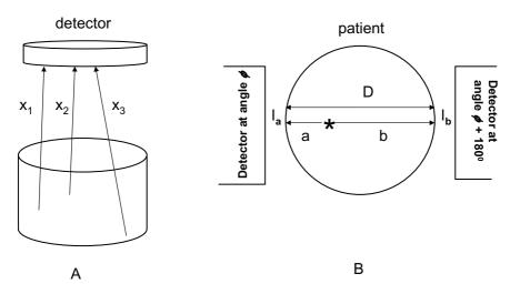
Fig. 12.16. **A.** Illustration of photons traveling different depths of tissue, thus suffering variable attenuation. **B.** Two photons traversing distances a and b are detected by the two detectors oriented at  $180^{\circ}$ . Attenuation correction can be applied by taking the geometric mean of the two counts  $I_a$  and  $I_b$  and using the total thickness D of the tissue in place of a and b separately.
