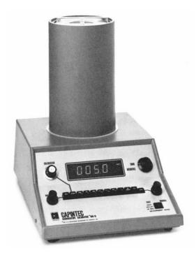
Fig. 7.3. A typical dose calibrator. (Courtesy of Capintec, Inc., Ramsey, NJ.)
