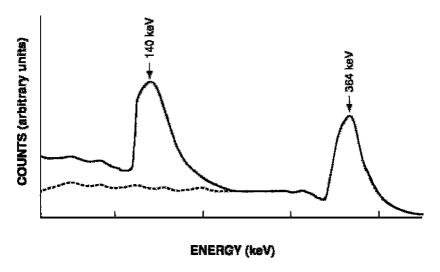
Fig. 8.12. A combined spectrum of the 140-keV  $\gamma$ -ray of  $^{99m}$ Tc and 364-keV  $\gamma$ -ray of  $^{131}$ I. The dotted line under the 140-keV photopeak is the spillover, or crosstalk, contribution from the 364-keV photon.
