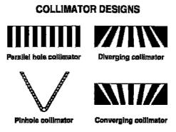
Fig. 9.3. Different designs of collimators.
