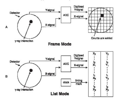
Fig. 11.2. Data acquisition in the frame mode and the list mode.
