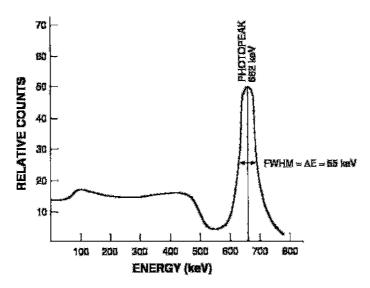
Fig. 8.7. The full width at half maximum (FWHM) of the 662-keV  $\gamma$ -ray of <sup>137</sup>Cs in a NaI(Tl) detector.
