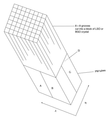
Fig. 13.1. A schematic block detector is segmented into  $8\times 8$  elements, and four PM tubes are coupled to the block for pulse formation. The pulses from the four PM tubes (A, B, C, and D signals) determine the location of the element in which 511-keV  $\gamma$ -ray interaction occurs, and the sum of the four pulses determines if it falls within the energy window of 511 keV.
