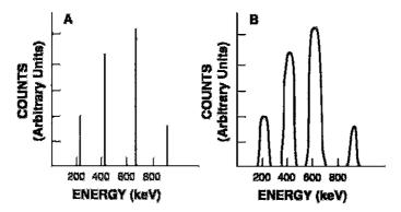
Fig. 8.2.  $\gamma$ -ray spectra. (A) An ideal spectrum would represent the different  $\gamma$ -rays as lines. (B) An actual spectrum showing the spread of the photopeak that is due to statistical fluctuations in the pulse formation.
