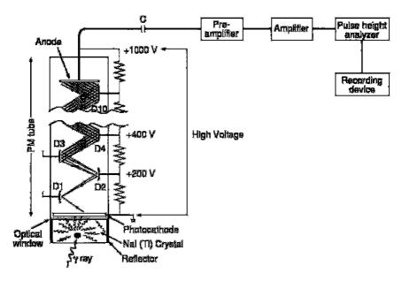
Fig. 8.1. A basic scintillation counter consisting of a NaI(Tl) detector, a photomultiplier (PM) tube, a preamplifier, a linear amplifier, a pulse-height analyzer, and a recording device. The high voltage applied to the PM tube is typically 1000 V.
