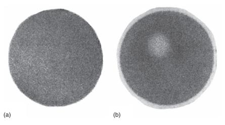
Fig. 10.9. Images of a <sup>57</sup>Co flood source showing the uniformity (a) and nonuniformity (b) of the response of a gamma camera.
