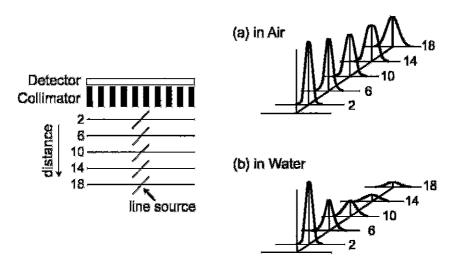
Fig. 10.5. Line spread function of a gamma camera equipped with a low-energy all-purpose parallel hole collimator obtained in (a) air and (b) water at different distances using a <sup>99m</sup>Tc-line source. Note that the resolution deteriorates in water due to attenuation.
