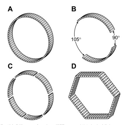
Fig. 13.2. Different configurations of PET scanners. (A) A circular full-ring scanner. (B) A partial ring scanner with a 15° angular shift between two blocks of detectors. (C) Continuous detectors using curve plates of Nal (TI). (D) Hexagonal array of quadrant-sharing panel detectors. (Reprinted with the permission of the Cleveland Clinic Foundation.)
