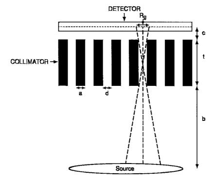
Fig. 10.1. A parallel-hole collimator with thickness t, hole diameter d, septal thickness a, and source-to-collimator distance b. The collimator is attached to a detector whose midplane is at a distance c from the back surface of the collimator.  $R_g$  is the collimator resolution.
