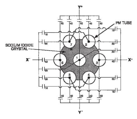
Fig. 9.4. Arrangement of seven photomultiplier (PM) tubes to produce X and Y pulses for the X, Y location of the  $\gamma$ -ray interaction in the detector.  $X^+$ ,  $X^-$ ,  $Y^+$ , and  $Y^-$  pulses are obtained by summing the output of all PM tubes weighted by capacitors for the location of each PM tube in relation to the site of  $\gamma$ -ray interaction. (Adapted from Anger HO. Scintillation camera. Rev Sci Instr. 1958; 29:27.)
