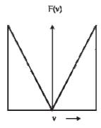
Fig. 12.8. The ramp filter in the frequency domain.
