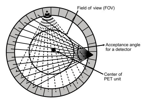
Fig. 13.4. The transverse field of view determined by the acceptance angles of individual detectors in a PET scanner. Each detector is connected in coincidence with as many as half the total number of detectors in a ring and the data for each detector are acquired in a "fan beam" projection. All possible fan beam acquisitions are made for all detectors, which define the FOV as shown in the figure. (Reprinted with the permission of the Cleveland Clinic Foundation.)
