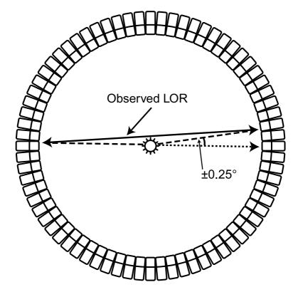
Fig. 13.13. Noncolinearity of 511-keV annihilation photons. Because there is some residual momentum associated with the positron, the two annihilation photons are not emitted exactly at  $180^{\circ}$ , but at a slight deviation from  $180^{\circ}$ . Two detectors detect these photons in a straight line, which is slightly deviated from the original annihilation line. The maximum deviation is  $\pm 0.25^{\circ}$ . (Reprinted with the permission of the Cleveland Clinic Foundation.)
