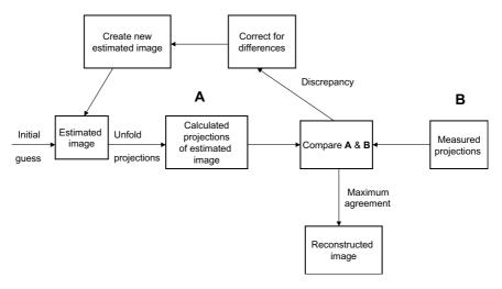
Fig. 12.12. Conceptual scheme of iterative reconstruction.
