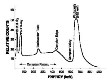
Fig. 8.3. A typical spectrum of the 662-keV  $\gamma$ -ray of <sup>137</sup>Cs illustrating the photopeak, Compton plateau, Compton edge, Compton valley, backscatter, characteristic lead K x-ray, and barium K x-ray peaks.
