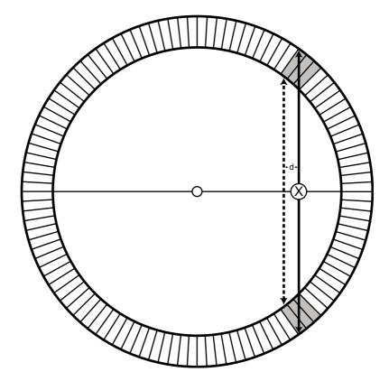
Fig. 13.11. An illustration of radial elongation. An off-center event (solid line) strikes the back of the detector pair tangentially. The X-, Y-positioning of the detectors (dashed line) is a distance d away from the actual location of the positron annihilation, causing the blurring of the image. (Reprinted with the permission of the Cleveland Clinic Foundation.)
