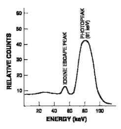
Fig. 8.4. A spectrum of 81-keV  $\gamma$ -ray of <sup>133</sup>Xe showing an iodine escape peak.
