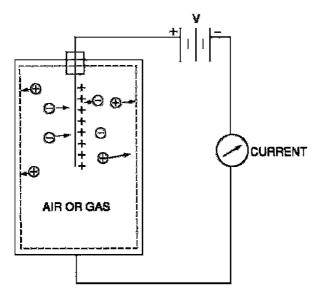
Fig. 7.1. A schematic diagram of a gas-filled detector illustrating the principles of operation.
