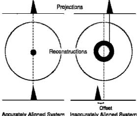
Accurately Aligned System Inaccurately Aligned System
