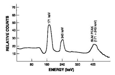
Fig. 8.5. A spectrum of <sup>111</sup>In with 171- and 245-keV photons showing a coincidence (sum) peak at 416 keV.
