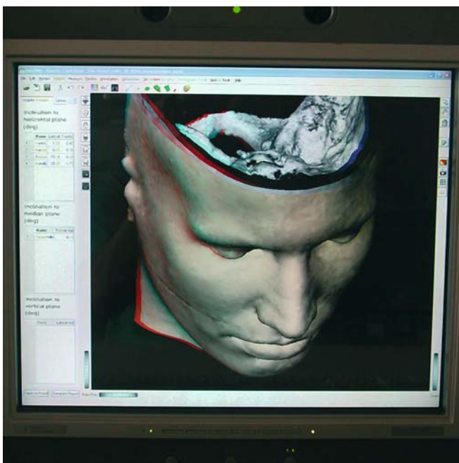
Fig. 10.11. Close-up view of auto-stereoscopic 3-D display (C-i display, www.seereal.com ) (3-D CT hard and soft tissue surface presentation, patient K.C.)
