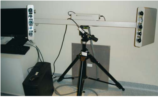
Fig. 10.7. Set-up of a commercial hardware system for 3-D surface imaging (3dMDface system, www.3dMD.com ) based on active stereo photogrammetry
