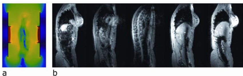
Figure 24. (a) B_1 field calculated for body-loaded, homogeneous, circularly polarized TEM volume coil at 300 MHz (7 T). (b) Sagittal images of human body at 7 T showing RF artifact predicted. Image acquisition parameters were: GE, TR/TE = 50/4 ms, matrix = 256^2 , thk = 3 mm, FOV = 35 \text{ cm}^2 , NT = 2, 55-sec scan. See attached CD for color version.
