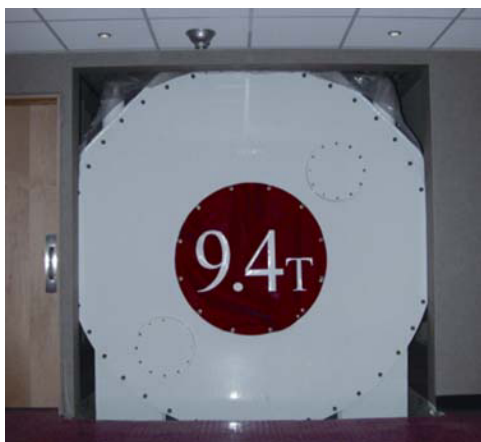
Figure 7. The 9.4T magnet in position in the iron magnet room just prior to closing the wall to cover all but the opening of the bore of the magnet (covered with red 9.4T sign). See attached CD for color version.
