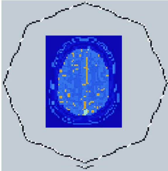
Figure 2. FDTD grid of the top circular ring of the birdcage coil. The different shadings on the grid correspond to different nonstandard FDTD algorithms used to achieve an accurate representation of the physical performance of the coil. These include lumped capacitors and slanted non-cubical cells for the curvatures of the ring as well as the struts. See attached CD for color version.
