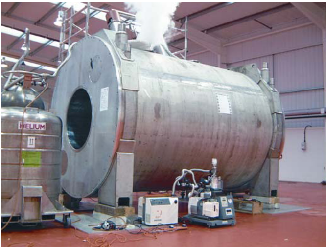
Figure 8. A 7T/900-mm bore magnet system in test. See the attached CD for the color version.
