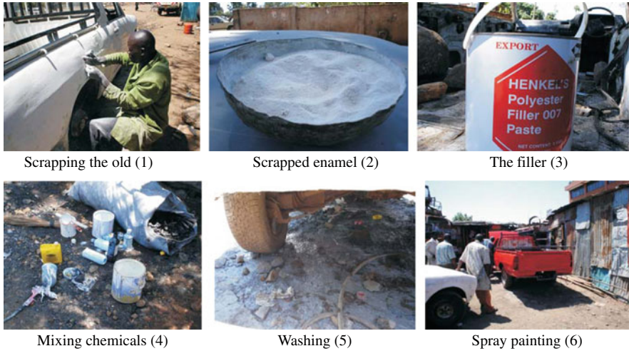
Fig. 15.8 The spray painting process and wastes in Kisumu (Kenya)
