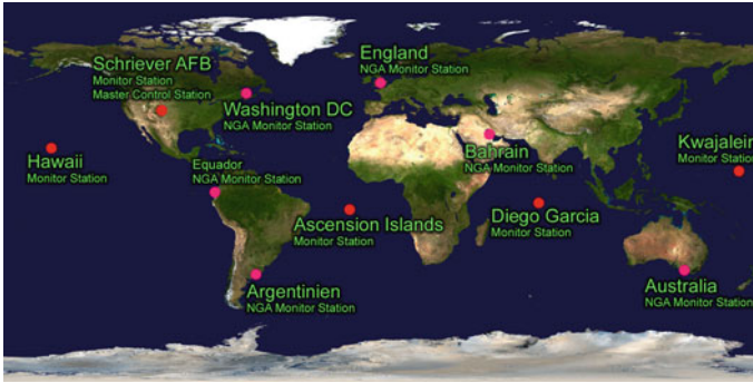
Fig. 3.2 GPS monitoring stations. Source http://www.kowoma.de/en/gps/control_segment.htm
