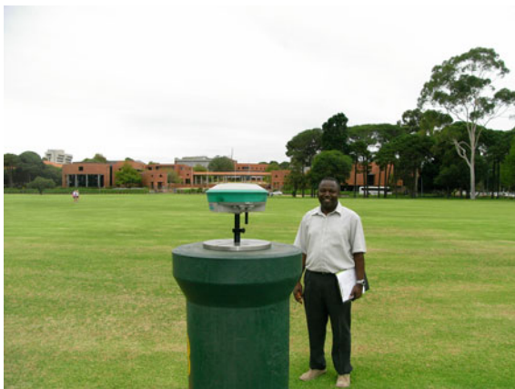
Fig. 5.5 Reference station, pillar 18 at Curtin University, Australia
