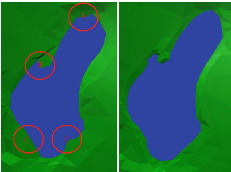
Fig. 8.7 Jack Finney Lake (September 2009). Left GNSS derived boundary. Right Total station derived boundary. The points marked on the left-hand figure are discussed in the text
