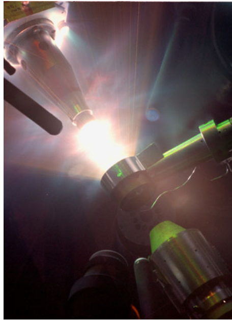
Fig. 3.8 Laser-driven shock-wave compression of a substance precompressed in a diamond anvil at the OMEGA facility [69].
