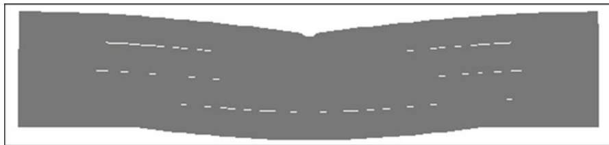
Fig. 3.10 Crack propagation in SBST simulation
