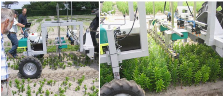
Fig. 25.5 Prototype canopy density sprayer for bed grown crops used in a lily crop; left in early growth stage with individual plants; right in late growth stage with fully covered bed
