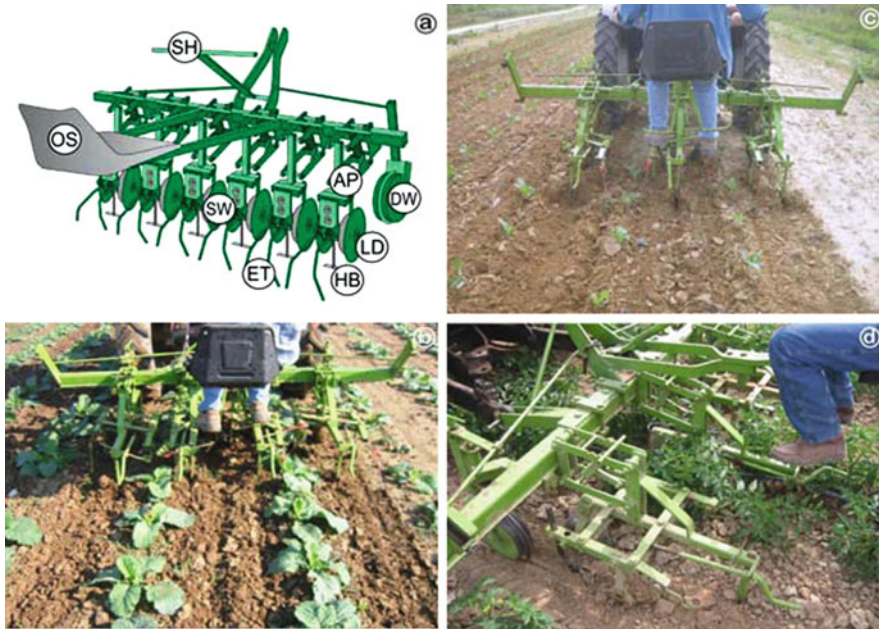
Fig. 17.7 Scheme of the precision hoe containing an operating seat (OS), steering handle (SH), articulated parallelogram (AP), directional wheel (DW), support wheel, lateral disc (LD), rigid elements with horizontal blade (HB) and elastic tines (ET) (a); precision hoeing in cabbage (b), in cauliflower (c), and in processing tomato (d). After (Peruzzi et al. 2007), courtesy images by Carlesi et al. (2009), Fontanelli et al. (2009), Raffaelli et al. (2009)
