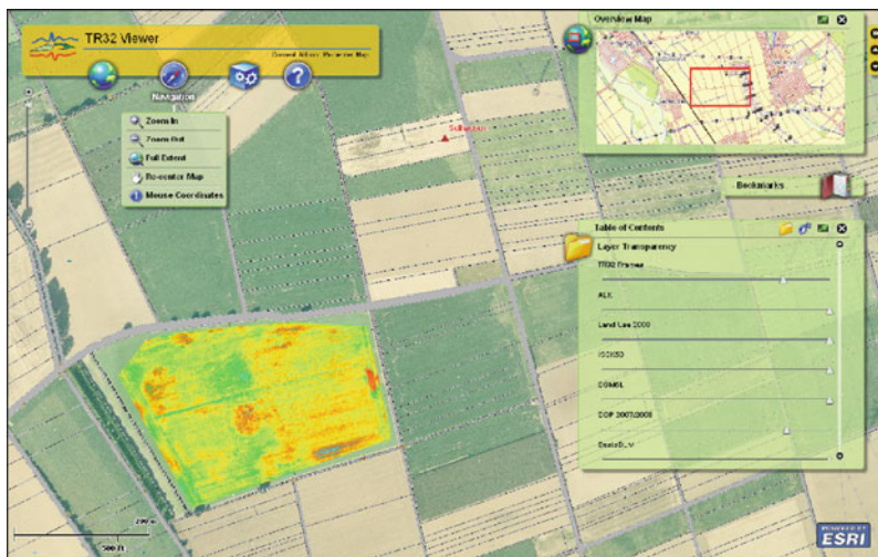
Fig. 13.8 WebGIS interface of the TR32 project ‘Soil-Vegetation-Atmosphere Patterns’: Aerial imagery (DOP), ALK, ATKIS, and for within-field variability of plant growth a plant height difference map of sugar beet from May to July 2008 obtained by terrestrial laser scanning (Hoffmeister et al. 2009, http://www.tr32db.de )
