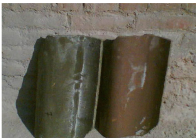
Fig. 8 Micro concrete roofing tiles made using chemical sludge
