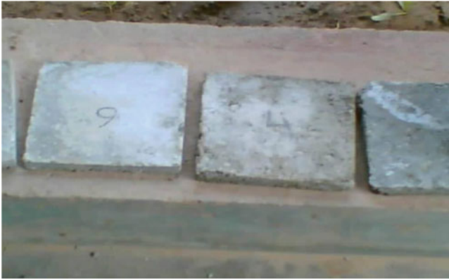
Fig. 9 Roofing tiles made using chemical sludge
