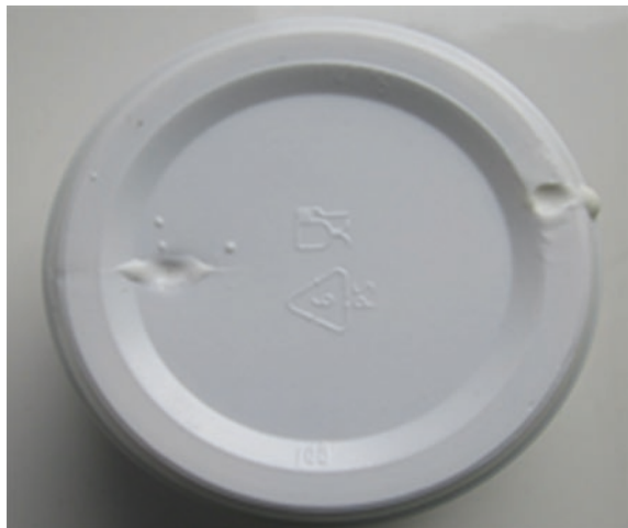
Fig. 5.3 Perforations in a PS container. Observed holes appear to exhibit roughly regular shapes
