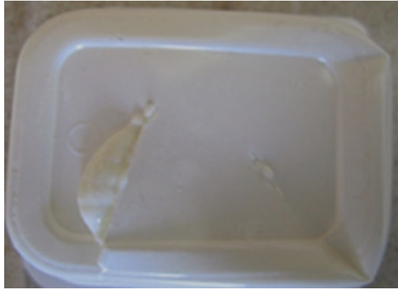
Fig. 5.2 Perforations in a PS container. Observed damages appear to exhibit irregular shapes
