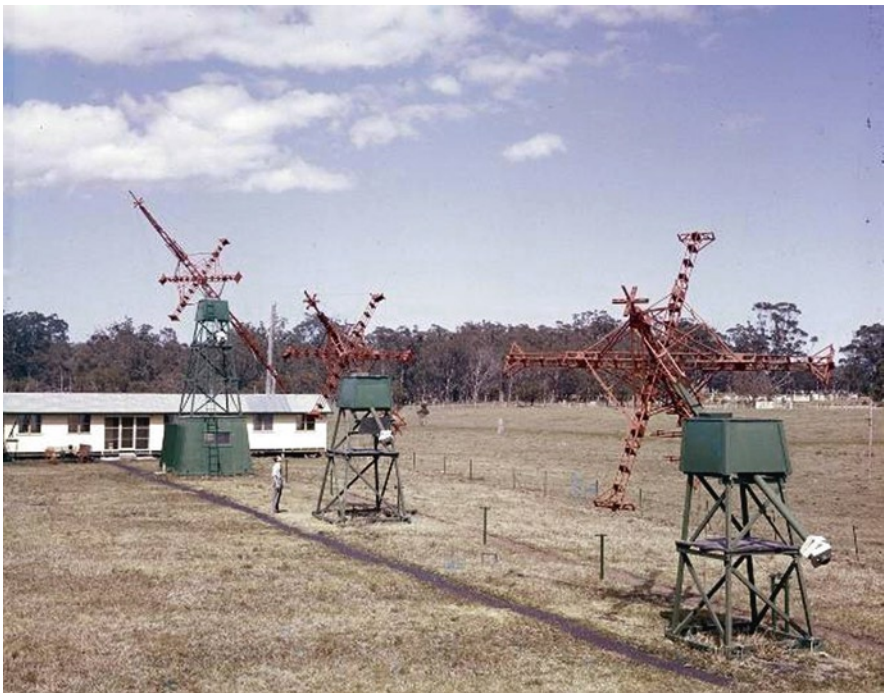
Fig. 5 The three crossed-rhombic aeriels of the 40–240 MHz Dapto Radiospectrograph (courtesy: ATNF Historic Photographic Archive).
