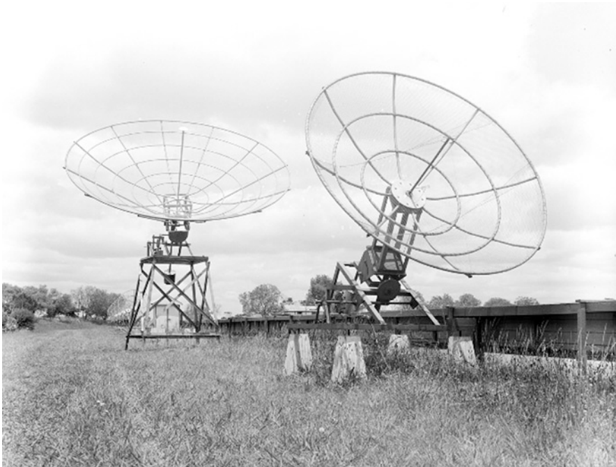
Fig. 28 On the left is a prototype of the larger aerial to be used in the new crossed array at Fleurs being tested at Potts Hill (courtesy: ATNF Historic Photographic Archive).
