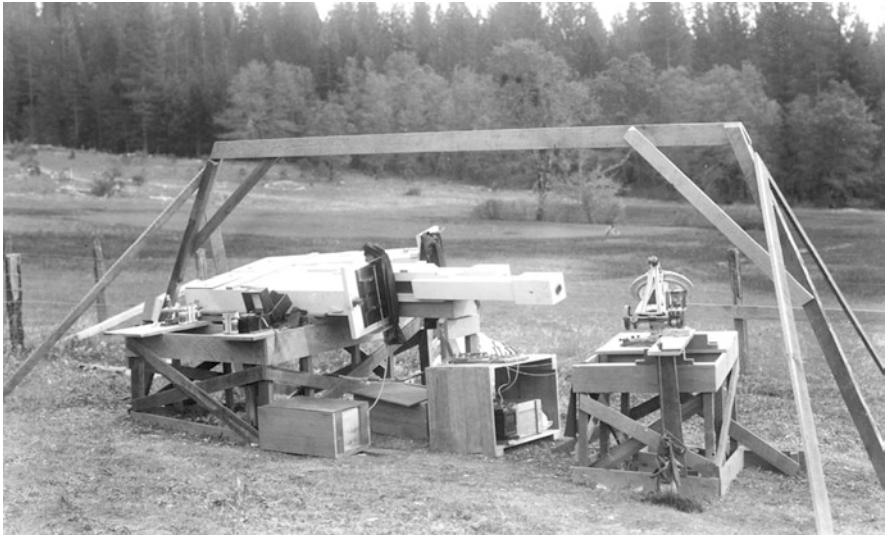
Fig. 8 Campbell's moving-plate spectrographs at the 1930 eclipse station (courtesy: Mary Lea Shane Archives of the Lick Observatory).
