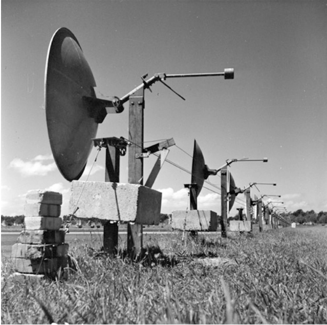
Fig. 14 The solar grating array in November 1951 on the southern bank of the Potts Hill No.1 reservoir (courtesy: ATNF Historic Photographic Archive: B2976-1).
