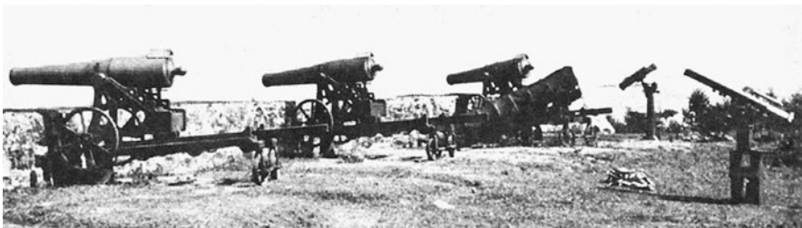
Fig. 19 The battery site at Cayenne in December 1889. The 18-in. reflector is mounted on the cannon carriage third from the left and part of the wooden tube can be seen in silhouette. The Clark refractor is located far right-center, and the Dallmeyer camera is immediately to the right of the reflecting telescope (courtesy: Mary Lea Shane Archives of the Lick Observatory).
