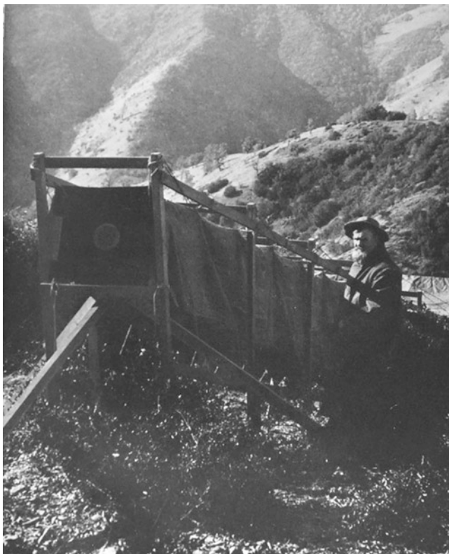
Fig. 5 The 40-ft Schaeberle Camera undergoing testing on Mt. Hamilton in 1892 (courtesy: Mary Lea Shane Archives of the Lick Observatory).
