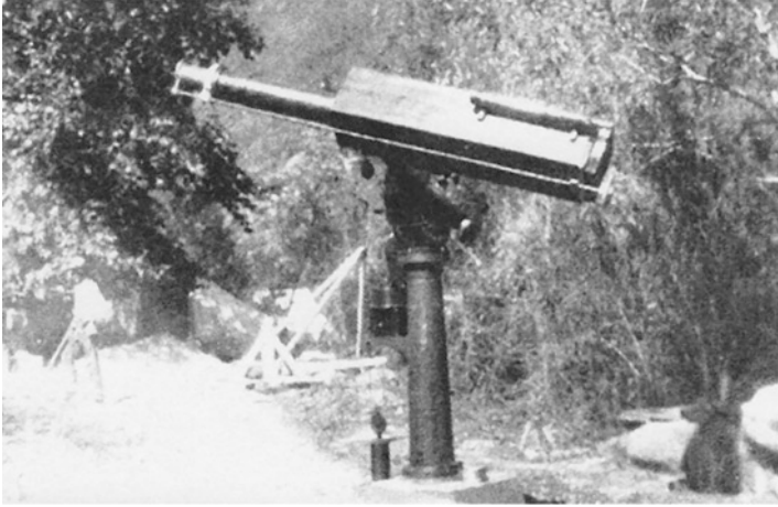
Fig. 7 The Floyd Camera on an equatorial mounting at the 1923 eclipse station (courtesy: Mary Lea Shane Archives of the Lick Observatory).
