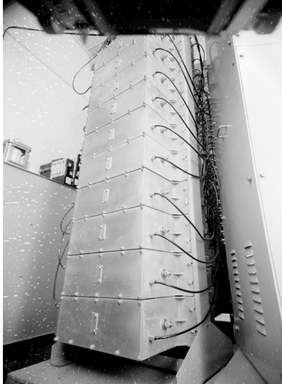
Fig. 9 The filters used in the Murraybank receiver (courtesy: ATNF Historic Photographic Archive B5985-1).
