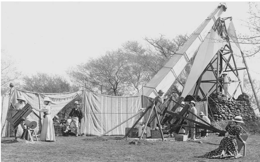
Fig. 26 The 40-ft Schaeberle Camera as Campbell redesigned it for the flat ground at Jeur. The plate-holder pit area is to the left and note the rock wall bracing the towers that support the Camera's tube and objective lens (courtesy of the Mary Lea Shane Archives of the Lick Observatory).
