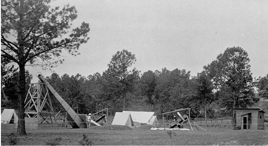
Fig. 30 View of the Thomaston eclipse camp. Note that the lower end of the Schaeberle Camera extends into a pit that was dug in the ground (after Campbell and Perrine 1900: 175).
