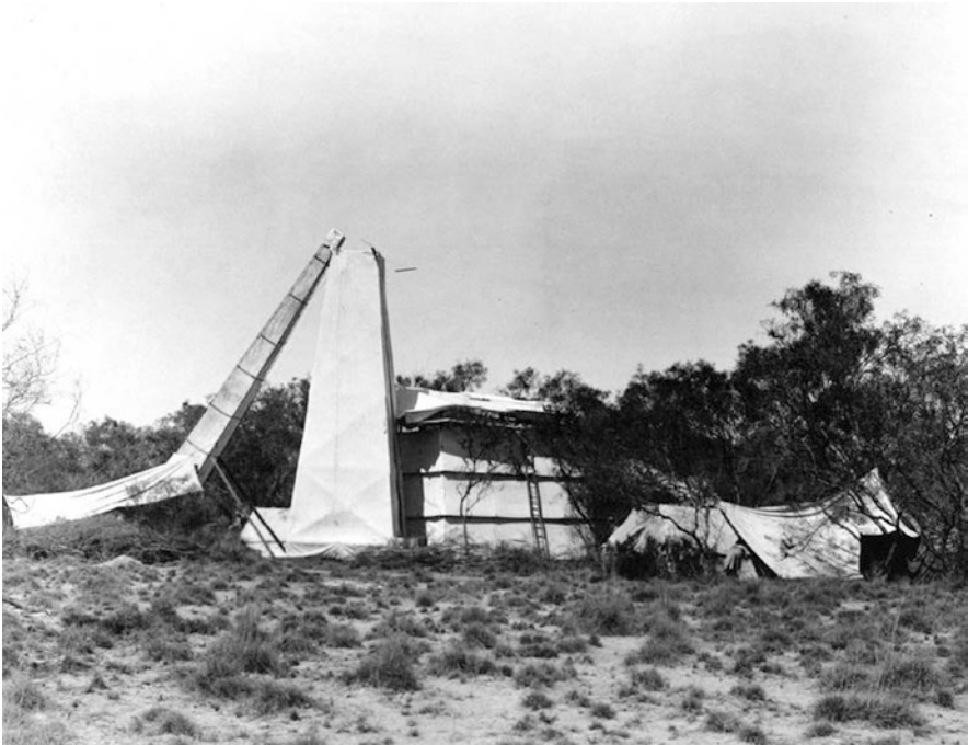
Fig. 50 White cloth was used to cover the 40-ft Schaeberle Camera, the Einstein instrument building and the tent at Wallal in 1922 (courtesy: Mary Lea Shane Archives of the Lick Observatory).
