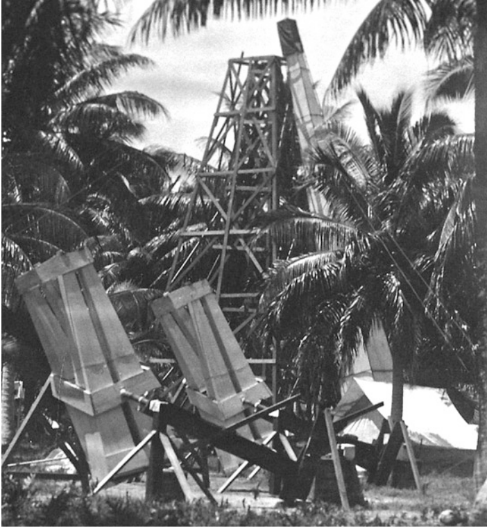
Fig. 41 The two 4-camera intra-Mercurial camera arrays in the foreground and the 40-ft Schaeberle Camera in the background among the palms at Flint Island in 1908 (courtesy of the Mary Lea Shane Archives of the Lick Observatory).
