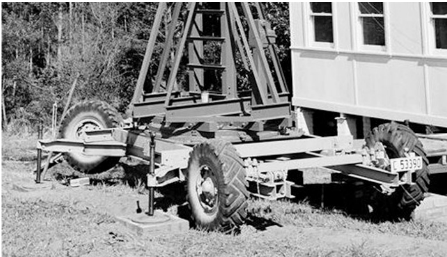
Fig. 3 The ex-British Army gun-laying 200 MHz radar trailer which was used for the alt-azimuth mounting of the Murraybank 21-ft aerial (adapted from ATNF Historic Photographic Archive B3973-1).
