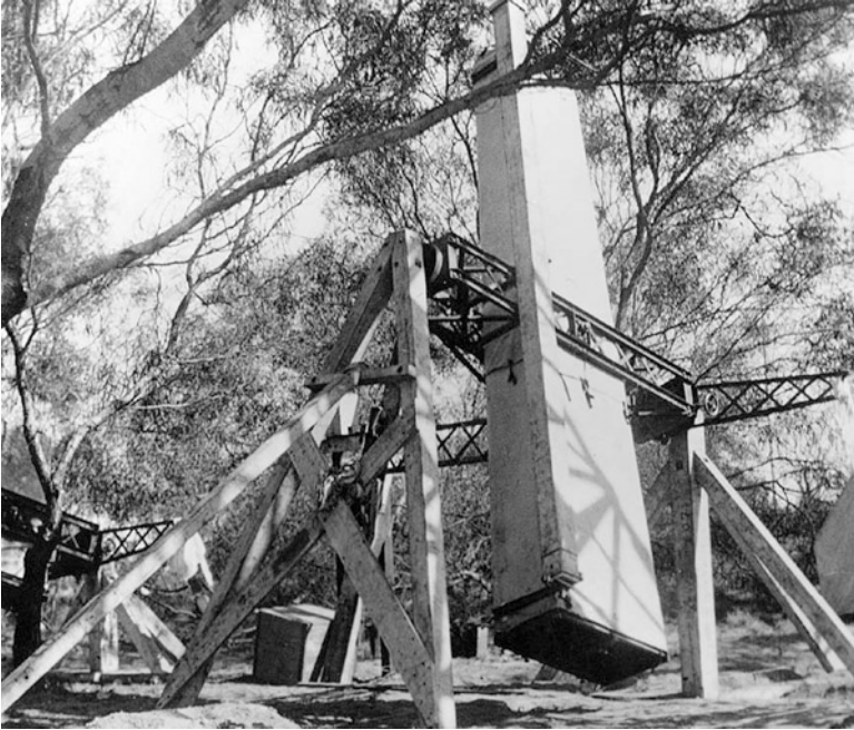
Fig. 52 The 15 foot focal length Einstein cameras with their guide telescope on a redesigned polar mounting of great stability (courtesy: Mary Lea Shane Archives of the Lick Observatory).
