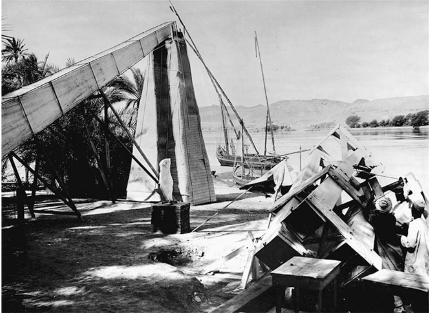
Fig. 38 The 40-foot camera is set up beside the Nile River at Aswan for the 1905 eclipse. The Vulcan cameras are in the foreground on the right (courtesy: Mary Lea Shane Archives of the Lick Observatory).
