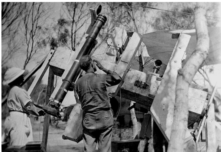
Fig. 51 The spectrographs and Floyd coronal camera. Mrs. Campbell has drawn the slide on the plate-holder of the Floyd camera (courtesy: Mary Lea Shane Archives of the Lick Observatory).
