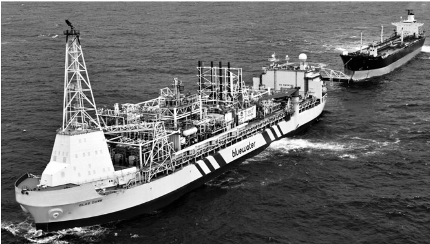
Fig. B.6 A floating production, storage and offloading (FPSO) ship on the left is connected to a tanker on the right. The FPSO ship processes and stores production from an offshore installation and off-loads periodically to tanker ships. (The image is courtesy of Bluewater Energy Services B.V., The Netherlands, www.bluewater.com )
