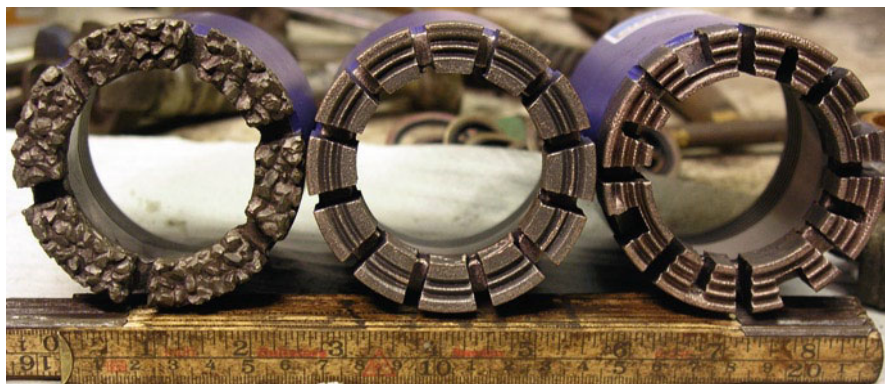
Fig. 4.6 From left : one tungsten carbide drill bit and two diamond-impregnated bits manufactured by Atlas Copco Craelius. (Source: Wikipedia)
