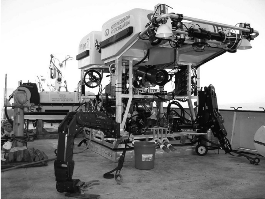
Fig. B.4 The Remotely Operated Vehicle (ROV) Hercules equipped with high-intensity lights at the top, a high-definition video camera in the center, and manipulator arms, including one arm with force feedback, giving an operator the “feel” of handling delicate specimens miles below the ocean’s surface. Similar ROV’s did most of the work necessary to secure the failed Macondo well. In routine operations, such ROV’s are used to construct and repair seafloor equipment and installations. Without them ultra-deepwater field operations would be impossible. (Source: NOAA, the photo is courtesy of Mystic Aquarium/IFE)
