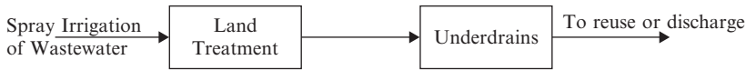
Fig. 15.7. Flow diagram of land treatment using slow rate system. (Source: US EPA (2)).
