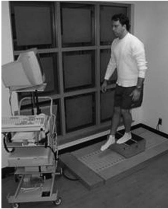
Fig. 16. Forward step-down test. The patient steps down an 8-in. step onto a forceplate (NeuroCom Balance Master System) as slowly and controlled as possible on each leg. Three trials are recorded. Mean impact and limb symmetry scores are calculated. Lower extremity control is observed for deviations. Normative data have established a mean impact of 10% body weight and limb symmetry of 85%.
