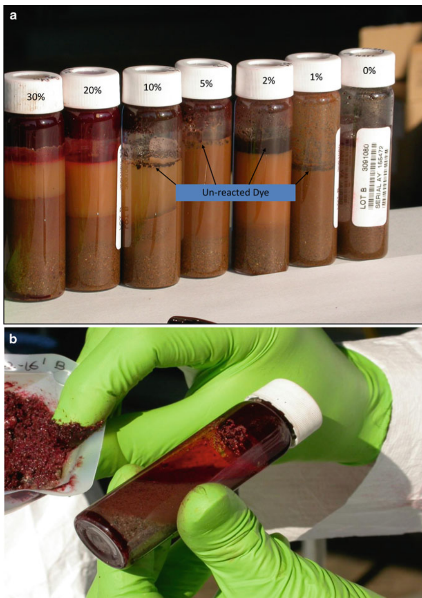
Figure 3.5. Hydrophobic dye testing using Sudan IV at the SRSNE Superfund Site, Southington, Connecticut. (a) Hydrophobic dye testing standards prepared using DNAPL and soil from the site. The percent number shown on the cap of the vial indicates the DNAPL saturation as a percentage of pore space. (b) Positive hydrophobic dye testing results at SRSNE in both a glass sample vial and a plastic dish ( left side of the figure ).
