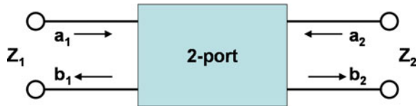
Fig. 2.28 A common 2-port with the symmetrical port notation
