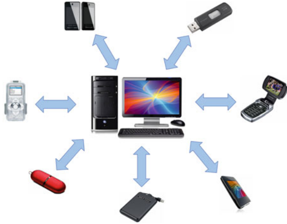
Fig. 1.4 Personal area network (PAN): a personal computer with portable devices like USB-sticks, mp3-players, mobile phones, etc. with typical data transmission distances of up to several meters
