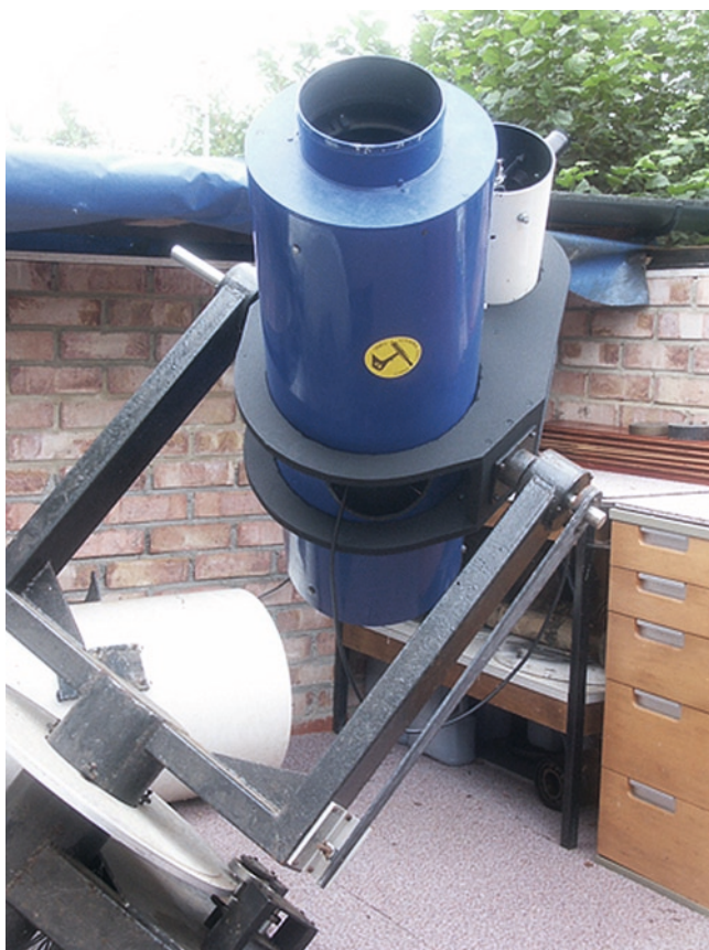
Fig. 12.8. The home made 160 mm f/2.5 Schmidt camera of Mike Harlow, as described in the text. Image: Martin Mobberley.
