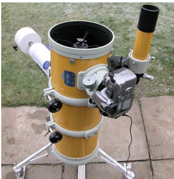
Fig. 12.2. A fast astrograph like Takahashi's 160-mm aperture f/3.3 Epsilon E-160 is ideal for comets, covering a degree or more of the sky. Image: Martin Mobberley.
