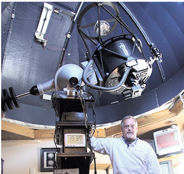
Fig. 15.7. Clay Sherrod of the Arkansas Sky Observatory is one of the world's most active comet imagers and astrometrists. He is pictured here with his 0.5-m PlaneWave CDK (corrected Dall-Kirkham) Cassegrain. Image: Clay Sherrod.
