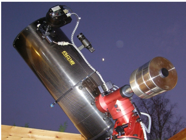
Fig. 15.4. Erik Bryssink's 0.4-m f/3.8 Orion Optics AG16 astrograph mounted on an Italian 10 \mu m GM2000 Qci mount at his run-off roof observatory in Kruibeke, Belgium. Image: Erik Bryssink.
