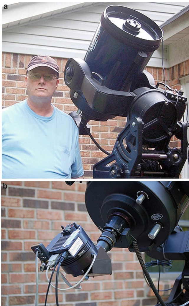
Fig. 15.9. (a) Charles Bell of Vicksburg, Mississippi is one of the world's most active comet imagers. Image: Charles Bell. (b) The business end of Charles Bell's 30-cm Schmidt-Cassegrain incorporates a focal reducer, an SBIG ST-8XME CCD, an SBIG AO-7 adaptive optics guider and an SBIG photometric filter wheel. Image: Charles Bell.
